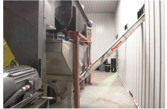
Explosive powder is transported from the ribbon blender and hopper by two flexible screw conveyors that are routed through the wall and rise 36 ft. (11 m) to a carousel that fills the Buttbuster tubes.
