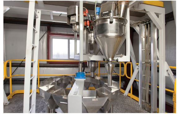
The rotating carousel (foreground) fills 12 Buttbuster tubes at a time, producing a 16.4 ft (5 m) length of explosive in seven seconds. The two flexible screw conveyors and hoppers feeding the carousel are visible in the rear.
