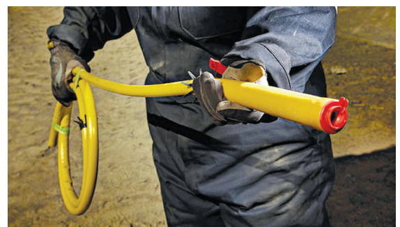
One-piece, custom-length Buttbuster tube creates a controlled blast by a precisely measured quantity of specially formulated explosive.
