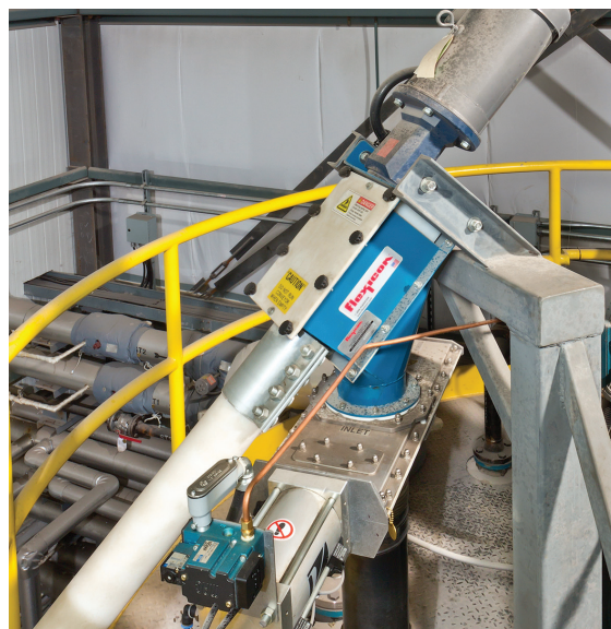
At the (blue) conveyor discharge, material exits prior to the point at which the flexible screw connects to gear reducer, preventing material contact with seals.
