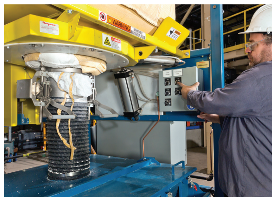
At the bag spout interface, a POWER-CINCHER® flow control valve regulates flow, while a SPOUT-LOCK® clamp ring and TELE-TUBE® telescoping tube promote complete, dust-free discharge.
