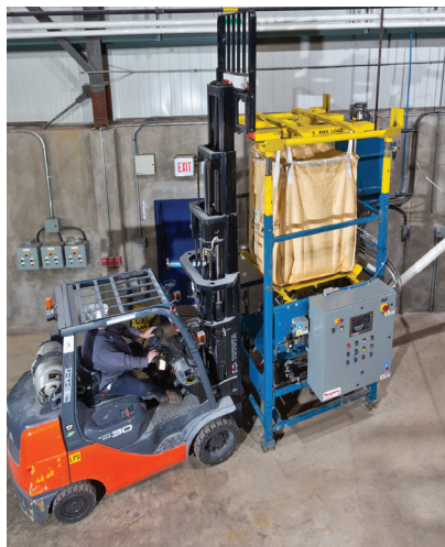
A lifting frame with bulk bag suspended, is forklifted into cradle cups at the tops of POP-TOP™ extension arms.
