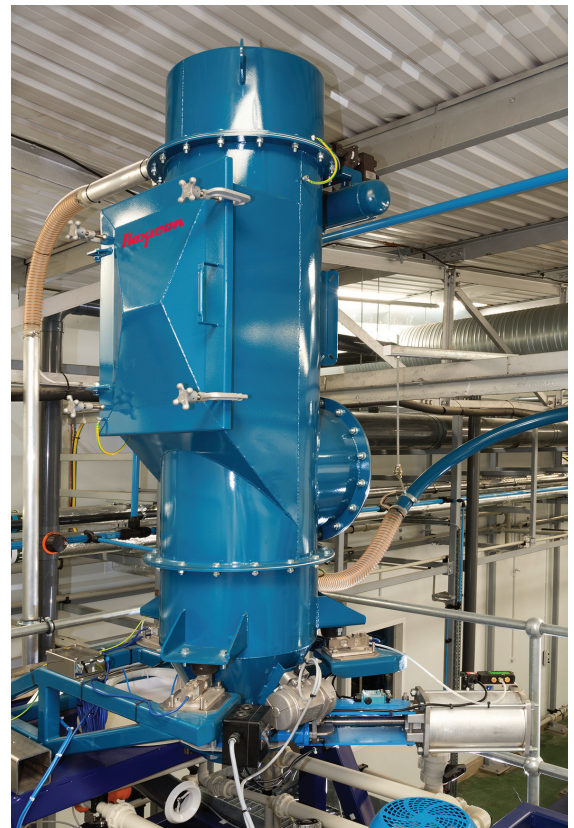
Powders move from the bag dump station through the pneumatic conveying line to the filter receiver (rear) in the main processing area. Fully enclosed system prevents the escape of dust.
