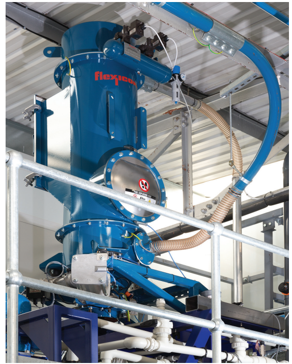
From the pneumatic line, the filter-receiver separates the silicon powder from the air stream before the powder enters the receiving hopper and is delivered to a slurry tank. A reverse pulse jet system cleans the filter cartridge at times intervals.
