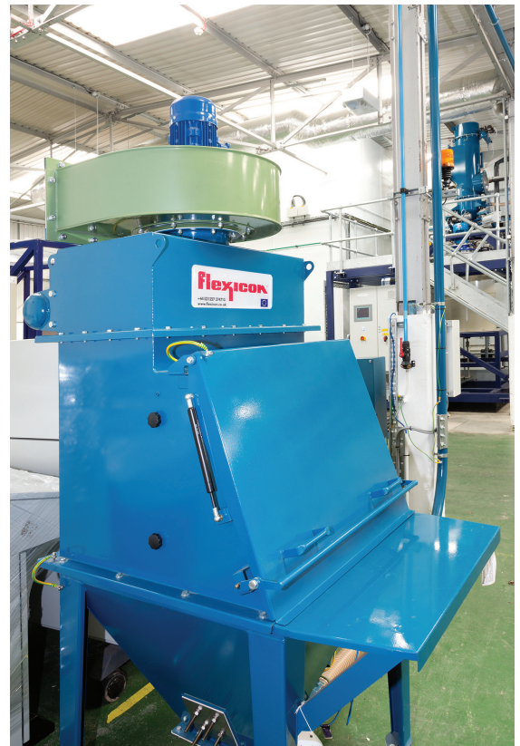
Powders move from the bag dump station through the pneumatic conveying line to the filter receiver (rear) in the main processing area. Fully enclosed system prevents the escape of dust.
