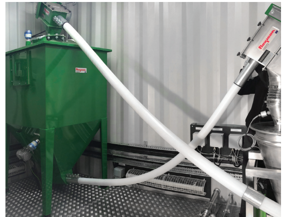
The 5 m long flexible screw conveyor (top left) moves the carbon powder from the bulk bag discharger to the green surge hopper.
