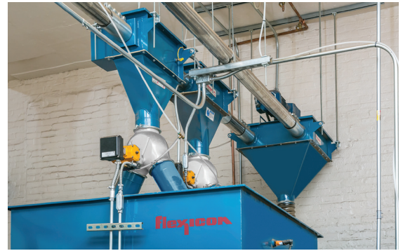
Each outlet from the TCC line connects to a wye diverter valve through which beans flow selectively into each bin of the four-bin hopper before beans enter the blender below.
