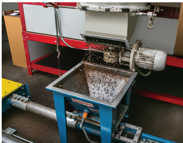
Beans discharge from the roaster into a hopper from where they are metered into the first tubular cable conveyor line.
