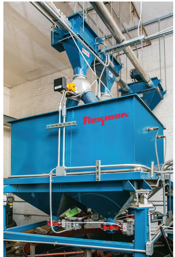
After loading from the roaster, the first tubular cable conveyor moves beans to a surge hopper for manual bag filling, or to two wye diverter valves (background), allowing selective discharging into a special four-bin hopper prior to blending.
