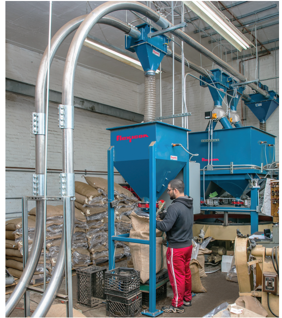
After loading from the roaster, the first tubular cable conveyor moves beans to a surge hopper for manual bag filling, or to two wye diverter valves (background), allowing selective discharging into a special four-bin hopper prior to blending.
