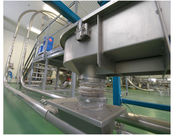
Oatmeal ingredients descend from the bulk bag discharger through a wire gate and vibratory feeder into the intake valve of the TCC circuit routed to the mixer.
