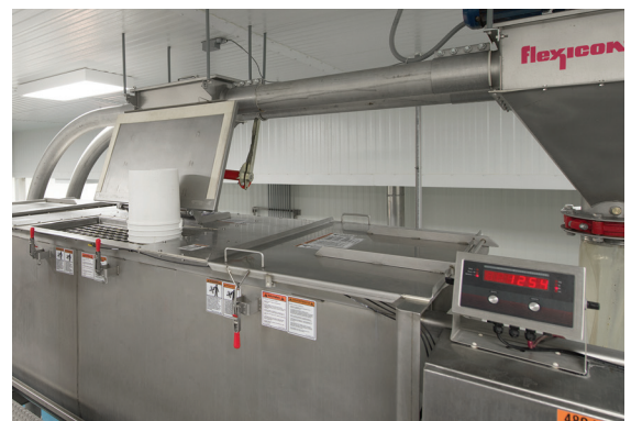
Granola ingredients flow from the TCC line through a full flow discharge adapter into the mixer.
