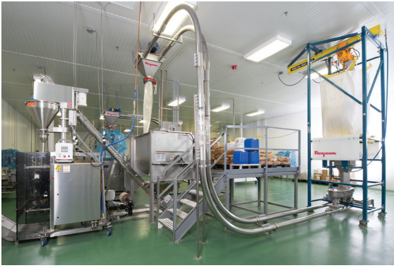
In the first oatmeal TCC circuit, ingredients from the cantilevered hoist style bulk bag discharger exit through a full flow inline discharge adapter into the mixer below. An inclined screw conveyor moves the mixed ingredients to a packaging machine (left).
