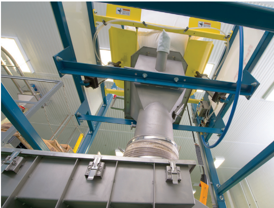
The first oatmeal TCC line, fed by a bulk bag discharger, is in the foreground. The second oatmeal TCC line, fed by a TIP-TITE® box dumper, is in the background.
