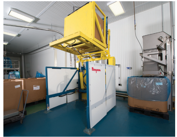
TIP-TITE® box dumper deposits contents of boxes of excess granola back into the TCC line to the packaging line.
