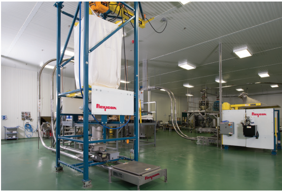
The first oatmeal TCC line, fed by a bulk bag discharger, is in the foreground. The second oatmeal TCC line, fed by a TIP-TITE® box dumper, is in the background.
