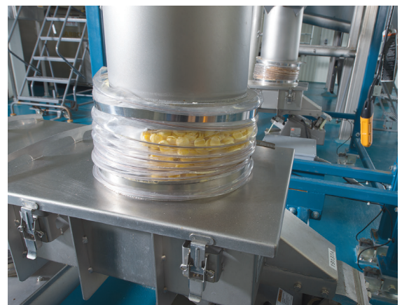
Minor granola ingredients are manually added to a hopper which discharges through a metered inlet adapter into the TCC line.
