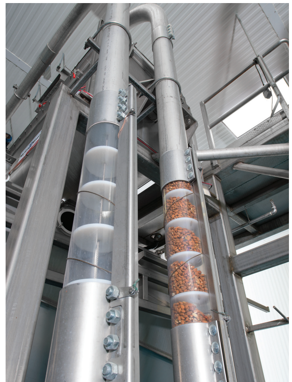
Transparent section of TCC circuit allows operators to observe system performance and fill level of "pockets."
