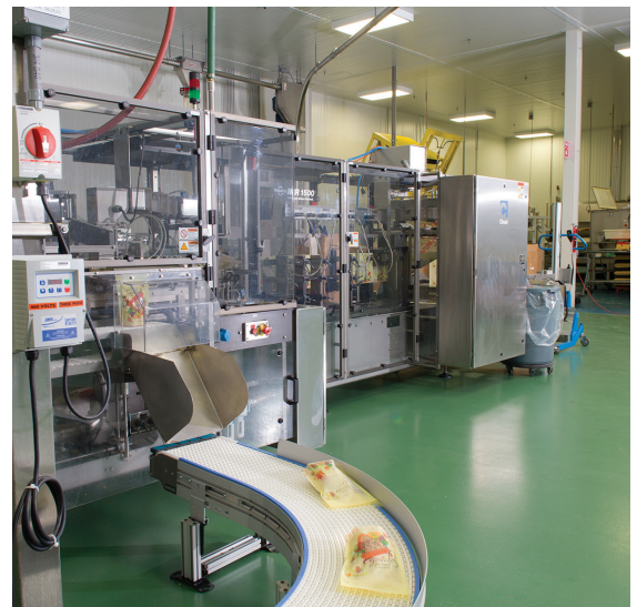
Packages of granola exit from the packaging machine.
