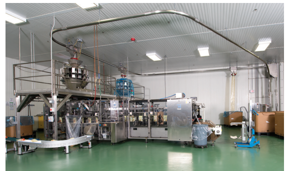
TIP-TITE® box dumper deposits contents of boxes of excess granola back into the TCC line to the packaging line.
