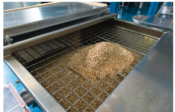
Granola tubular cable conveyor circuit: Minor ingredients are manually added through hopper at right while major ingredients are metered from two bulk bag dischargers into the tubular cable conveyor that feeds the mixer (background).
