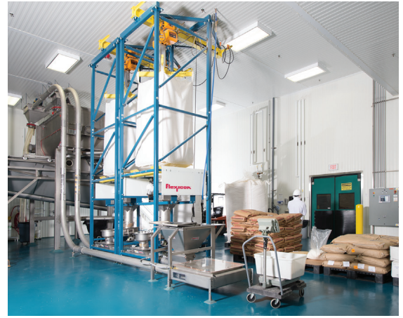
Granola tubular cable conveyor circuit: Minor ingredients are manually added through hopper at right while major ingredients are metered from two bulk bag dischargers into the tubular cable conveyor that feeds the mixer (background).
