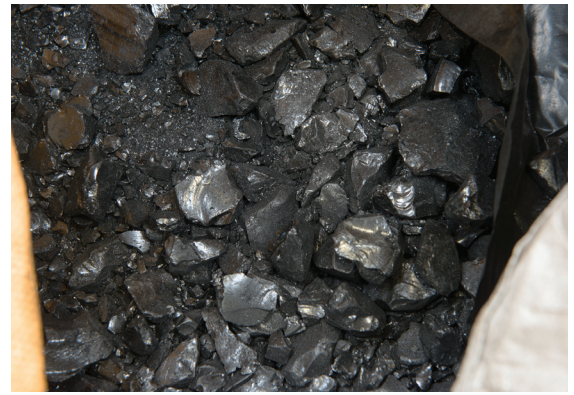
Raw pitch solidifies during the shipment and must be reduced to a size that can freely discharge from the bulk bag.
