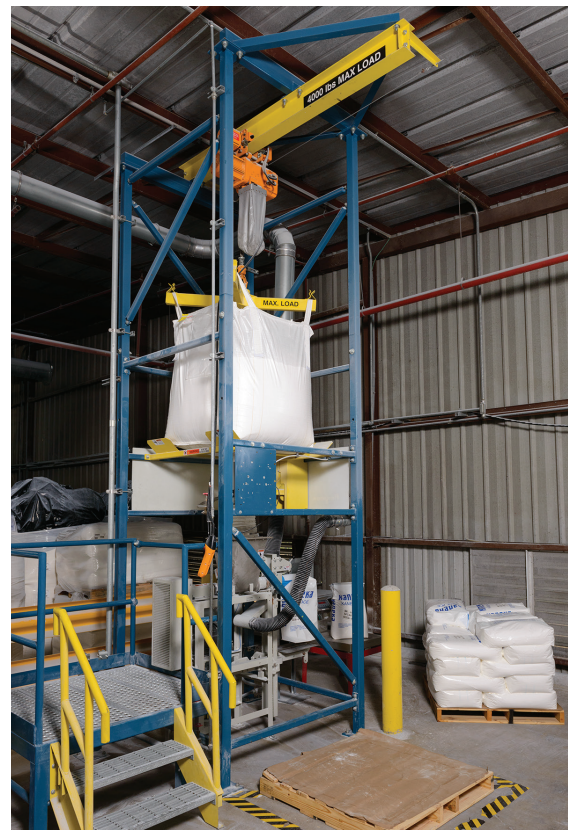
'Bulk-to-sack' system: The bulk bag is loaded into the frame using the discharger's cantilevered I-beam, electric hoist and trolley, and then gravity discharged through the telescoping tube into a filling machine for 50 lb (23 kg) sacks.
