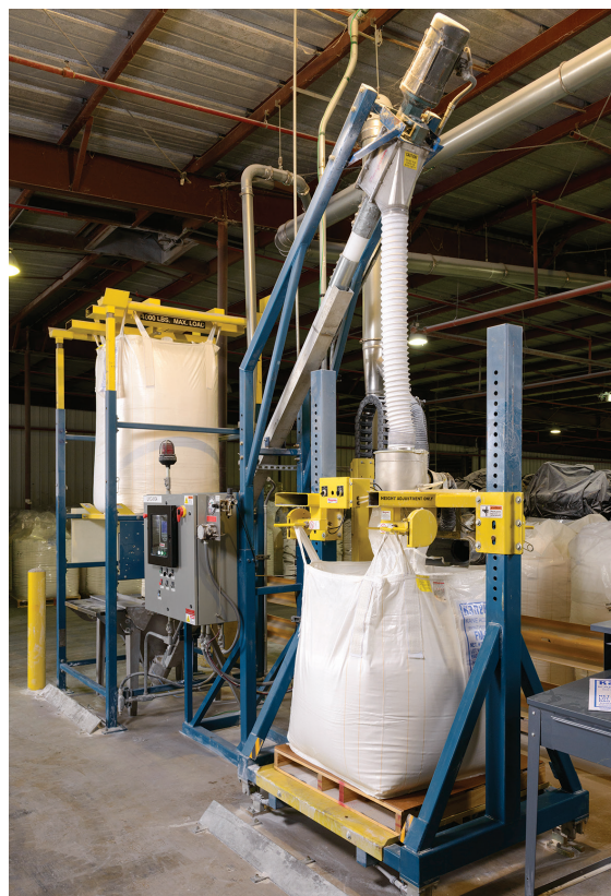
The flexible screw conveyor transfers material from the bulk bag discharger (rear) to the bulk bag filler (foreground). A height-adjustable fill head accommodates bulk bags in any of three sizes used by the company.
