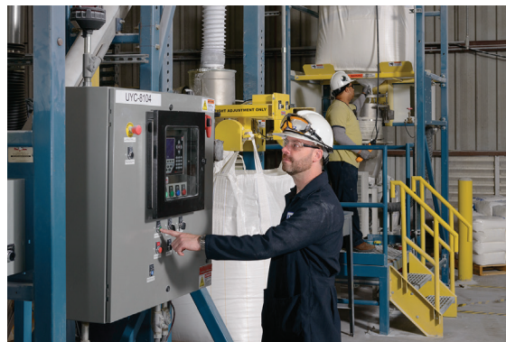
Operator in foreground initiates a bulk bag filling cycle while operator in background loads a bulk bag into the discharger frame using its electric hoist and trolley.
