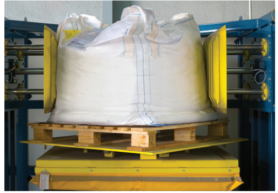
Hydraulic rams fitted with specially contoured end plates press opposite sides of the bag to loosen solidified powders. The turntable and bag rotate 90° to condition all sides, while the scissor lift allows conditioning at all heights.
