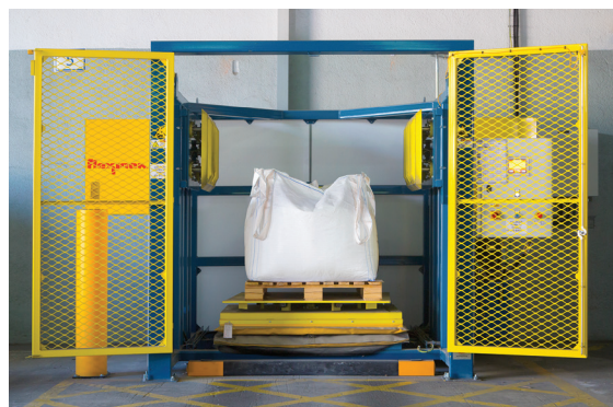
Once the safety doors are secured, the operator initiates the conditioning cycle.
