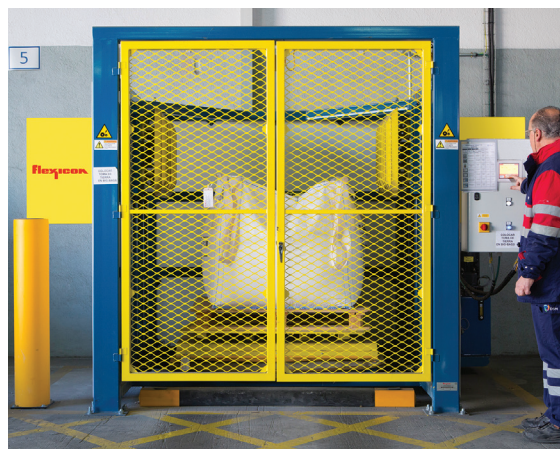
Once the safety doors are secured, the operator initiates the conditioning cycle.
