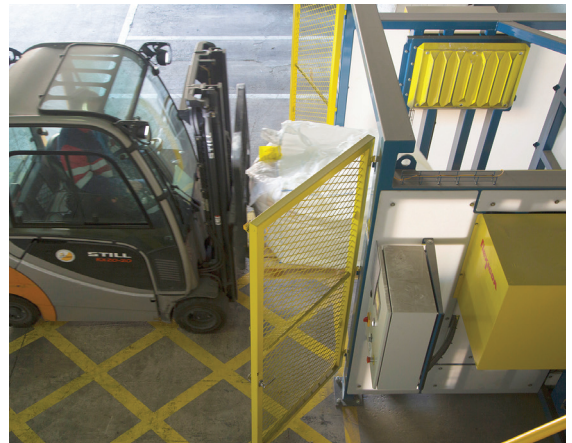
Forklift moves a bulk bag from the conditioner to a reactor.
