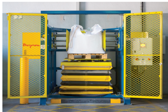
Scissor lift raises the bulk bag to a preselected height while hydraulic rams with contoured end plates press opposite sides of the bag to loosen solidified powders.
