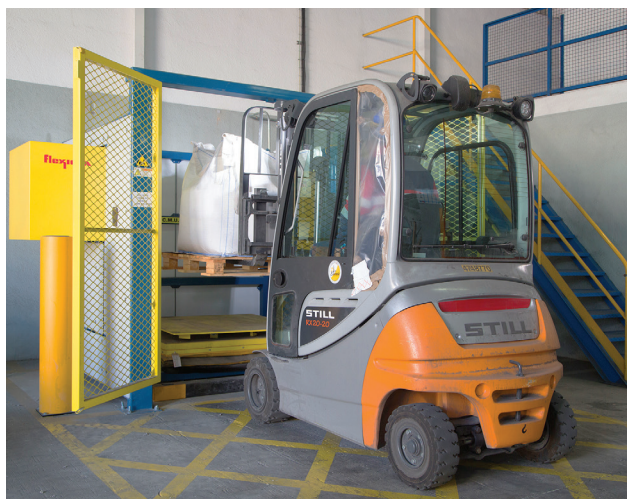
Forklift loads a bulk bag into the conditioner
