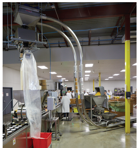
Overall view of third tubular cable conveyor line shows the hopper and intake at the tensioning wheel end (left), the conveyor's horizontal and vertical 'S' shape, and discharge at the drive wheel end (right) into the cup packaging line.
