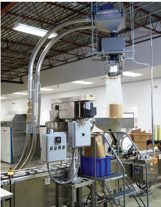
Tubular cable conveyor curves to vertical and discharges at the drive wheel end into the cup packaging line.
