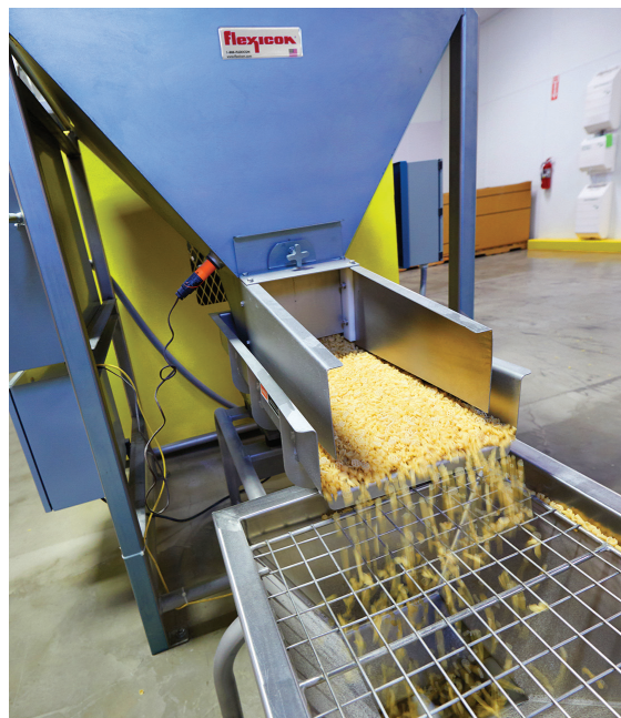
Open-Chute Box Dumper empties a Gaylord into the large hopper from which pasta moves on a vibratory tray feeder into the smaller hopper and inlet adapter of the Flexi-Disc® tubular cable conveyor.
