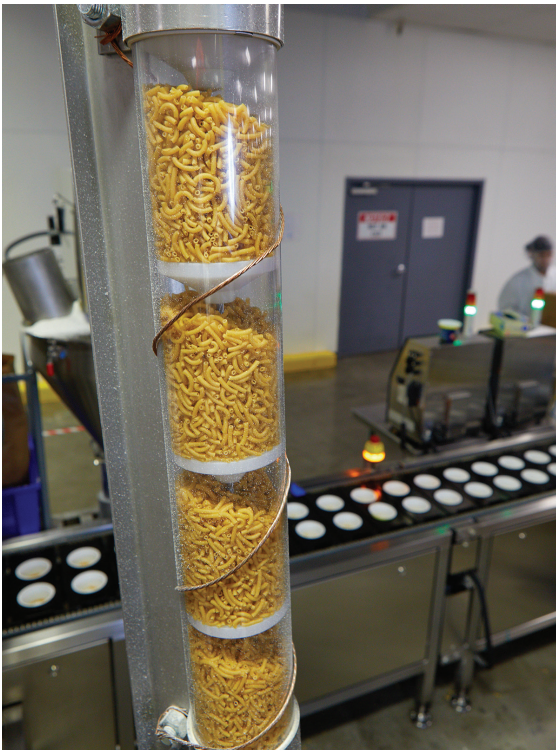
A clear section of vertical tubing permits visual monitoring of system performance and product quality during transport.
