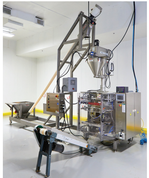
Portable "cheeser" line includes a 5.5 cu ft (156 l) hopper and 15 ft (4.6 m) long Flexicon screw conveyor for packet packaging of cheese powder.
