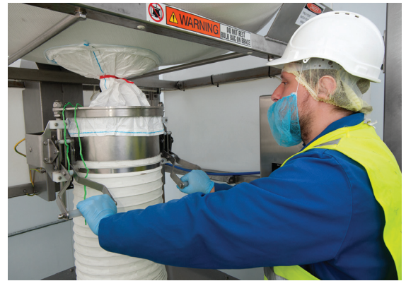
Once the bag spout is secured by a SPOUT-LOCK™ clamp ring, the operator releases the drawstring (red). Constant downward tension is maintained by a TELE-TUBE™ telescoping tube as the bag empties and elongates.
