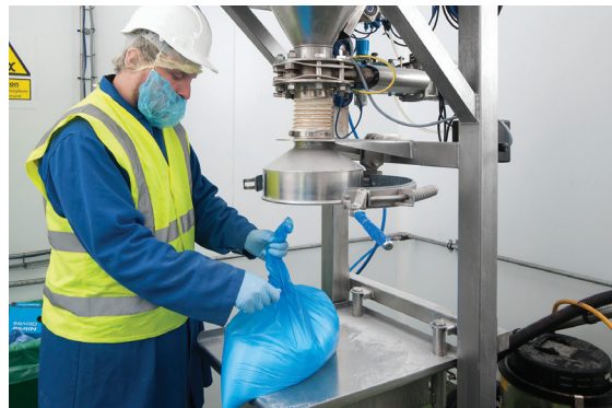
Operator ties off and removes filled 10 kg plastic bag for storage.
