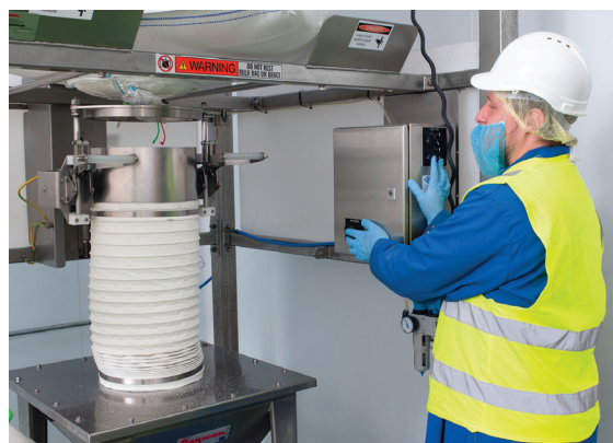
Here, the operator pneumatically raises the TELE-TUBE™ telescoping tube prior to securing the bag spout using a SPOUT-LOCK™ clamp ring.
