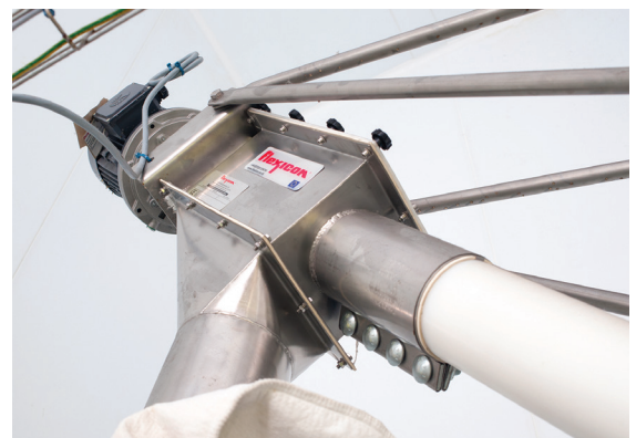
The flexible screw conveyor is driven beyond the point at which sugar is discharged, preventing material contact with bearings or seals.
