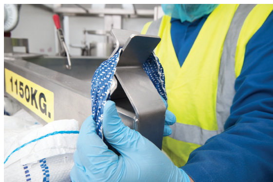
Operator attaches strap to one of four Z-CLIP™ bag strap holders before the lifting frame and bag are hoisted and rolled into the discharger.
