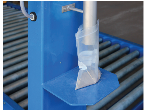
A pneumatically-operated product sampler captures a 4.3 oz (142 g) specimen from the material stream for product quality documentation.
