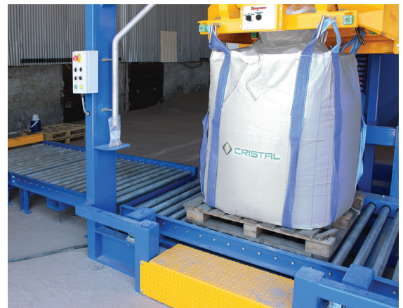
The Swing-Down® fill head pivots to a vertical position, allowing the operator to safely and rapidly attach bag straps to filler latches while standing on the plant floor. Pushing one button inflates the material inlet against the bag spout, and initiates all automatic bag filling functions.
