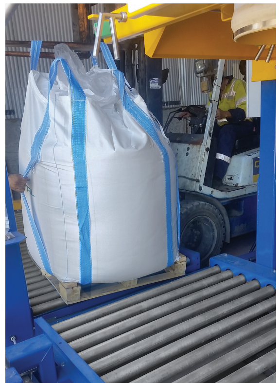
The filled bag and pallet move out on the roller conveyor and are removed for shipment.
