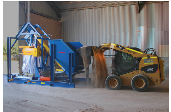
The automated bulk bag filling station fills bulk bags with up to 352,000 lb (160,000 kg) of abrasive materials per eight-hour shift.
