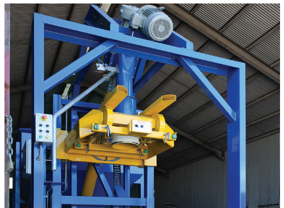
Skid-steer loader deposits mineral sands into the 88 ft 3 (2.5 m 3 ) capacity hopper while the screw conveyor moves the material to the bulk bag fill head.
