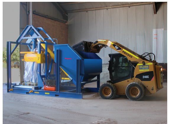
Skid-steer loader deposits mineral sands into the 88 ft 3 (2.5 m 3 ) capacity hopper while the screw conveyor moves the material to the bulk bag fill head.
