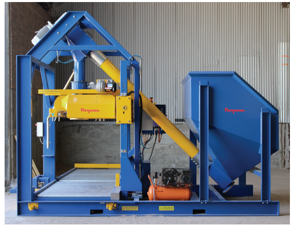
The automated bulk bag filling station fills bulk bags with up to 352,000 lb (160,000 kg) of abrasive materials per eight-hour shift.
