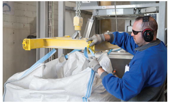
Operator delivers bulk bag, and attaches bag loop straps to the lifting frame.
