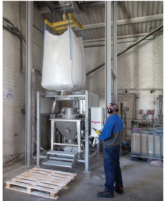
The cantilevered hoist and trolley position the bag for discharge into the 226 L hopper and through a rotary valve into the pneumatic line.
