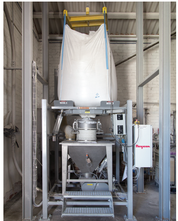
The powder flows dust-free into the hopper and into the 38 m long pneumatic transfer line.
