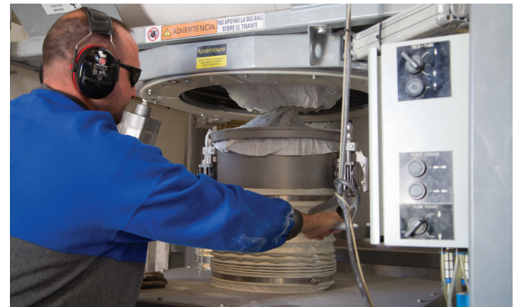
Next he connects the spout to a Spout-Lock® clamp ring, which is mounted on a Tele-Tube telescoping tube that promotes material flow and eliminates dust.
