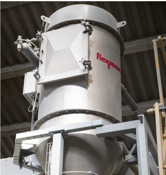
From the pneumatic line, the filter-receiver separates the mineral powder from the air stream before discharging the powder into the extruder. System operation is under PLC control.
