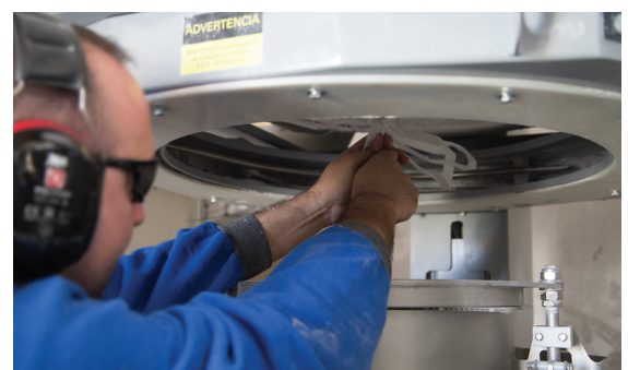
The operator pulls the bag spout through the Power Cincher® flow control valve which prevents product leakage and facilitates tying off a partially-empty bag.
