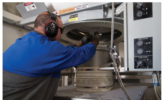
The cantilevered hoist and trolley position the bag for discharge into the 226 L hopper and through a rotary valve into the pneumatic line.
