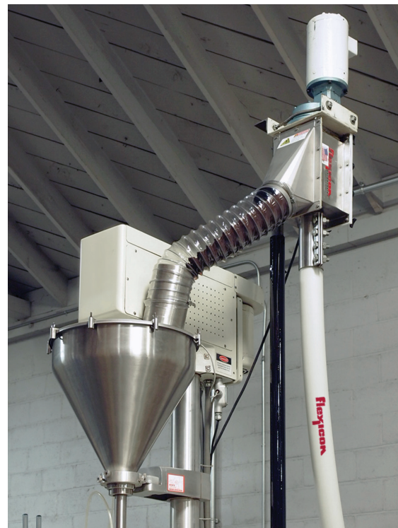
A flexible spiral is the only moving part contacting the coffee, which is discharged below the point at which the spiral connects to the drive motor, preventing material contact with seals or bearings.
