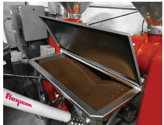
The 8 cu ft (226 l) capacity hopper and cover are fabricated of stainless steel with sanitary finish.
