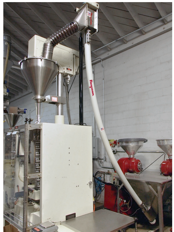
The 8 cu ft (226 l) capacity hopper and cover are fabricated of stainless steel with sanitary finish.
