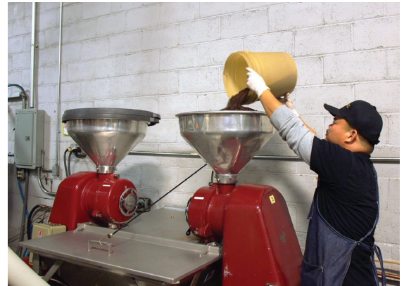
Coffee is discharged from two grinders into the 8 cu ft (226 l) capacity hopper that charges the flexible screw conveyor.
