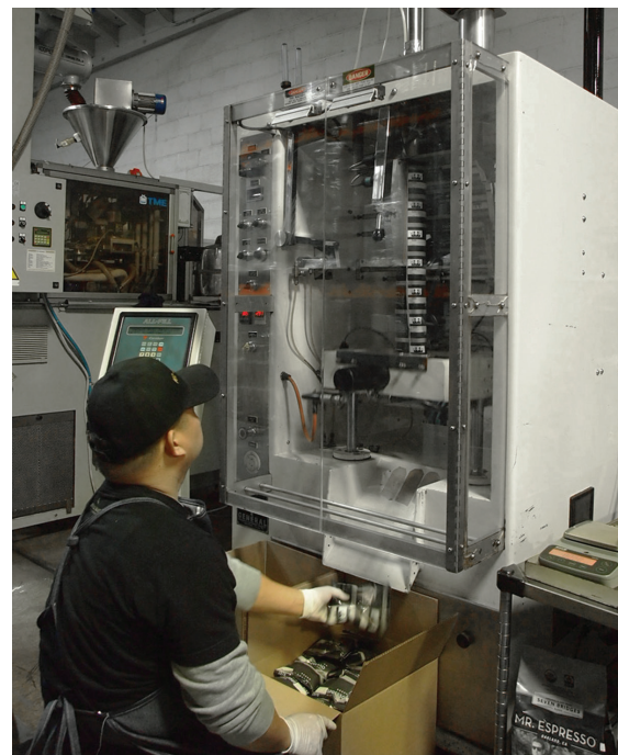
A flexible spiral is the only moving part contacting the coffee, which is discharged below the point at which the spiral connects to the drive motor, preventing material contact with seals or bearings.
