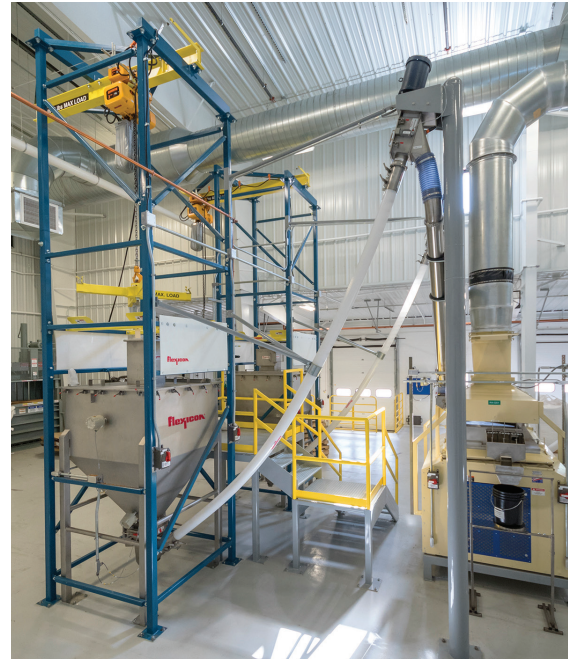
Side-by-side beam-and-hoist style bulk bag dischargers allow for one frame to discharge material while the other is reloaded.
