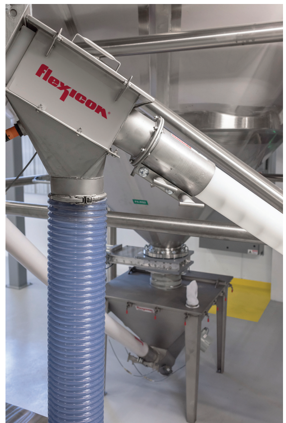
The motor sits forward of the flexible screw conveyor discharge, preventing material contact with seals or bearings.
