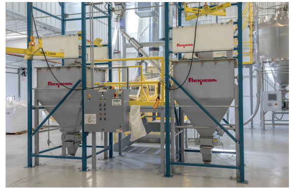
Side-by-side beam-and-hoist style bulk bag dischargers allow for one frame to discharge material while the other is reloaded.
