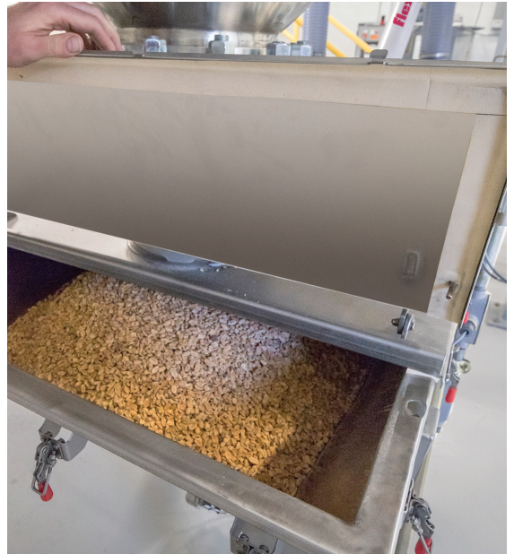
The hinged lid on the hopper permits manual inspection.
