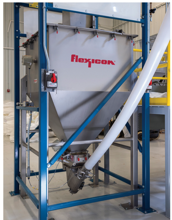
From the hopper of each discharger, a flexible screw conveyor transports raw peanuts to the gravity separator.
