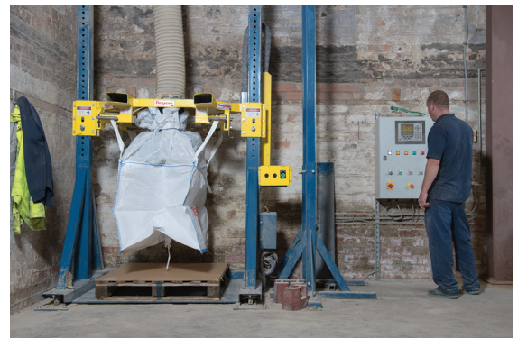
With the bag inlet secured to the downspouting, the automated weigh-filling cycle is initiated.
