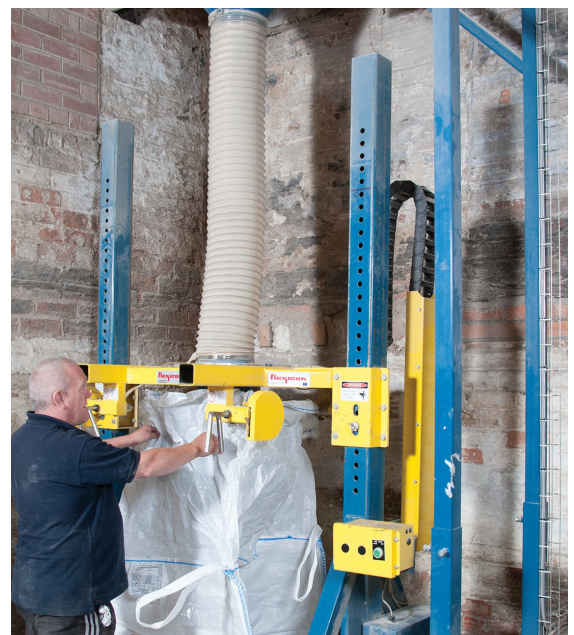
Bag spout is connected before malt is transferred from a silo through a horizontal flexible screw conveyor and downspouting into the bulk bag filler inlet.
