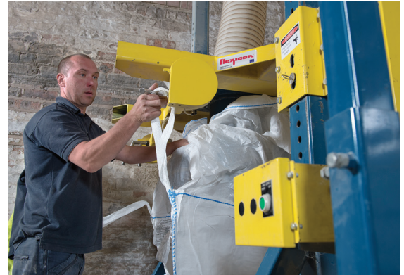
Operator attaches bag loops to the four retractable bag hooks on the fill head.
