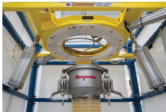
Operator pulls the bag spout through the Power-Cincher™ flow control valve in which four elliptically contoured bars cinch the bag spout concentrically, enabling partially emptied bulk bags to be retied and removed.
