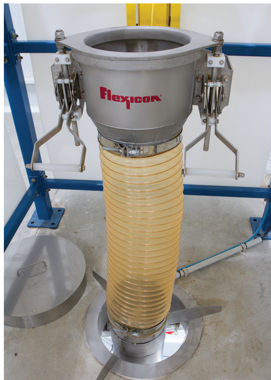
The Spout-Lock™ clamp ring creates a sealed connection between the clean side of the bag spout and the clean side of the Tele-Tube™ telescoping tube, which raises the clamp ring for connection to the bag spout and then lowers, applying continual downward tension to promote flow into packaging machine on the floor below.
