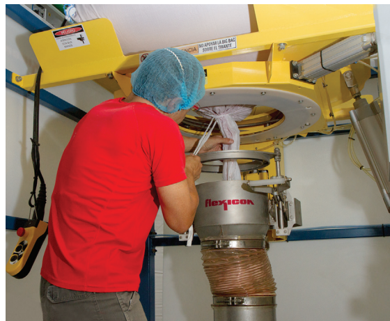
Seven Bulk-Out® model BFC-C-X half-frame bulk bag dischargers feed 70 tonnes per day to packaging machines on the floor below. An electric hoist positioned over each discharger lifts the bag onto the half frame.
