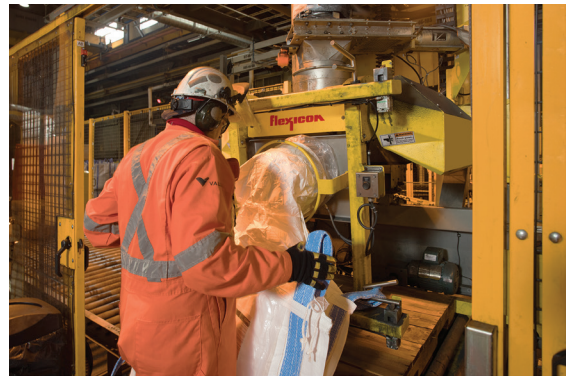
Each bulk bag filler features an articulated Swing-Down fill head, allowing the operator to safely access all bag connection points from floor level. Load cells measure weight gain of the bag, allowing a PLC to stop filling the bag once it reaches target weight.
