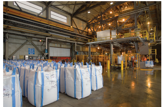
The automated bulk bag filling system includes two bulk bag fillers (rear), a central pallet dispenser, and two 25 ft (7.5m) long roller conveyors from which a fork truck offloads filled bags for shipment.
