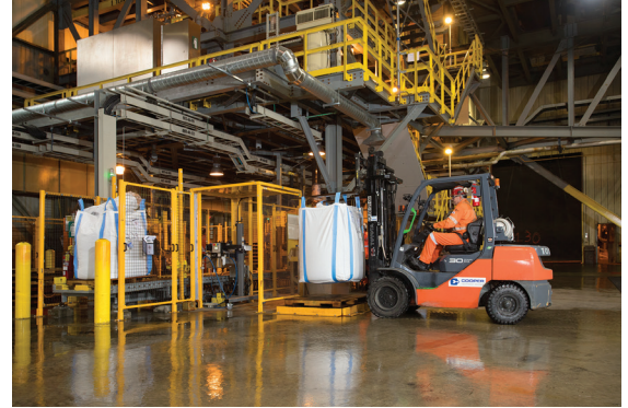
Filled bulk bag is removed from holding bin at the end of the 25 ft (7.5m) long roller conveyor.
