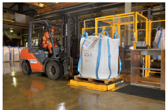
Automated pallet dispenser (right) feeds pallets to the bulk bag filler which receives copper concentrate granules from the 11 ton (10 m.t.) capacity hopper above.
