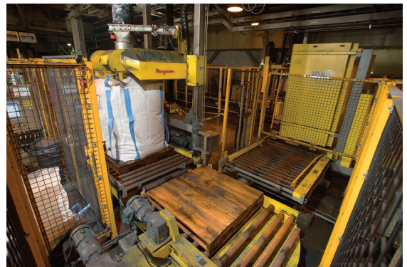
Automated pallet dispenser (right) feeds pallets to the bulk bag filler which receives copper concentrate granules from the 11 ton (10 m.t.) capacity hopper above.
