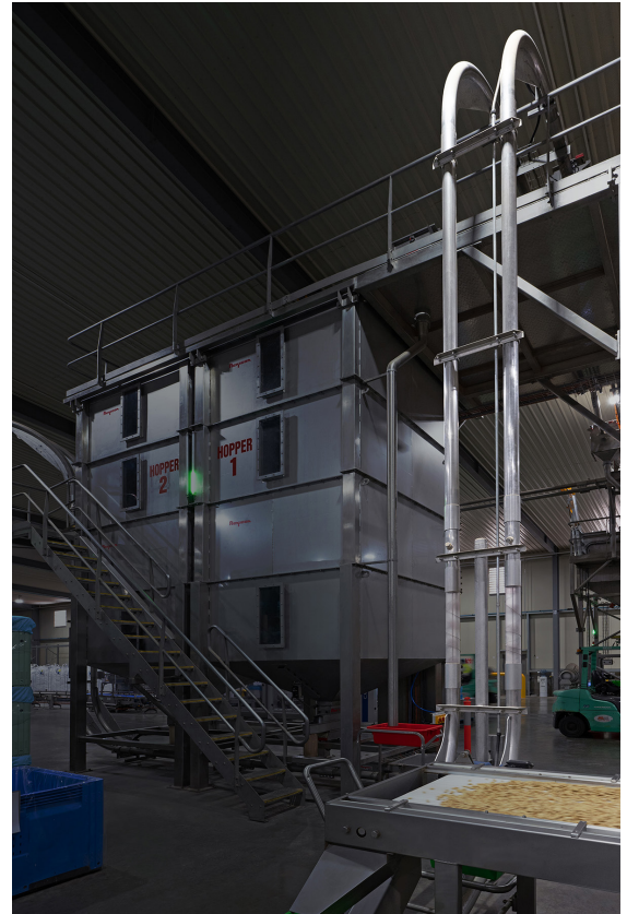
This FLEXI-DISC® tubular cable conveyor system climbs horizontally over 12m to reach the top of the twin storage hoppers servicing slicing and packaging operations.
