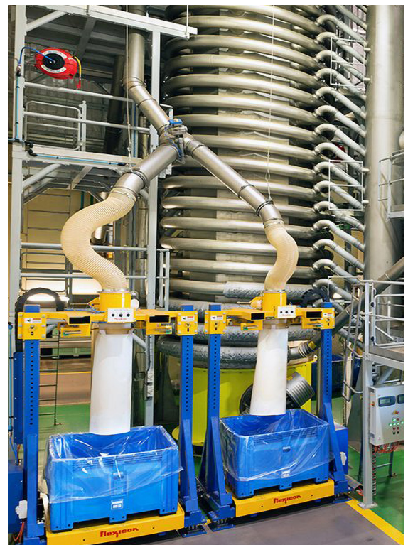
Flexicon's TWIN-CENTERPOST™ bulk bag fillers are already known for their ability to fill bulk bags, but their adaptability is further showcased through a modification that allows them to fill rigid totes. (source: Almondco)
