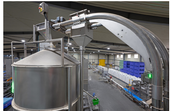
In the foreground, a Flexi-Disc System feeds a storage silo, while in the background, filled bulk bags of whole blanched almonds are prepared for shipment to Almondco's consumer product processors.
