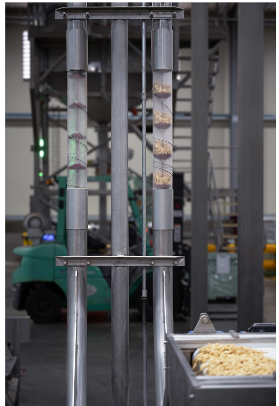
This FLEXI-DISC® System gently conveys the fragile whole blanched almonds from the blancher towards downstream processing functions.
