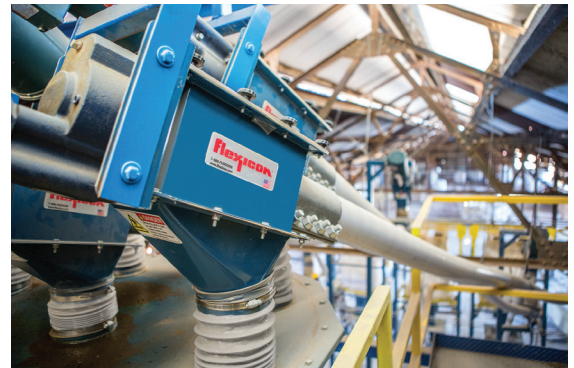
The operator pulls the bag spout through the iris valve and closes the valve before untying the bag spout and closing the access door. The valve is opened gradually to prevent bursts of material and dust.
