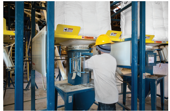
The operator pulls the bag spout through the iris valve and closes the valve before untying the bag spout and closing the access door. The valve is opened gradually to prevent bursts of material and dust.
