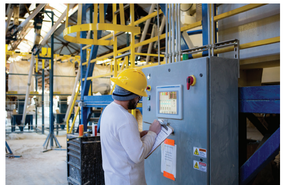
Programmable controls enable operators to vary bulk bag discharging, conveying, weighing, and mixing on a batch-by-batch basis. An HMI includes options for automatic or hand-mode operation, as well as set points, adjustments, status, start/stop, completion and other parameters.
