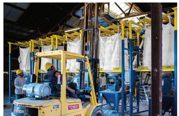
A fork truck inserts the lifting frame holding the bulk bag into receiving cups atop the discharger frame.
