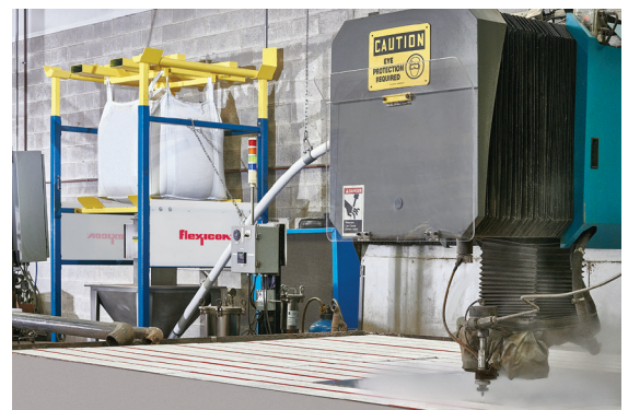
Garnet delivery system allows uninterrupted operation of the water jet cutter for maximum production without dusting, spillage or worker fatigue, while reducing material costs.
