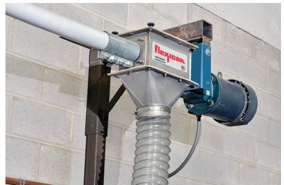
The conveyor screw is driven beyond the point at which garnet exits the conveyor, preventing contact with seals or bearings.
