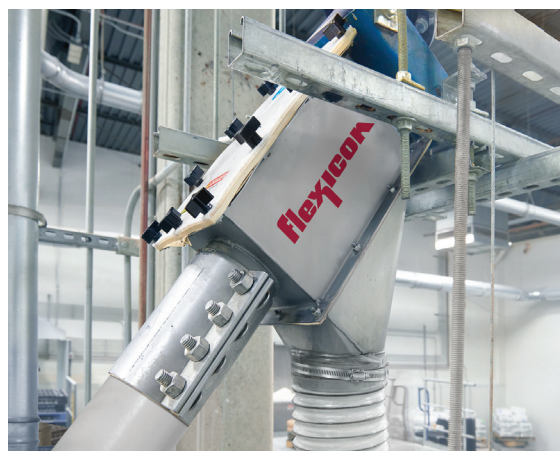
Material exits the conveyor below the point at which it is driven, preventing contact with seals or bearings.
