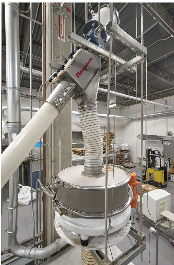
Material discharged from the flexible screw conveyor is screened before being fed to a packaging machine.
