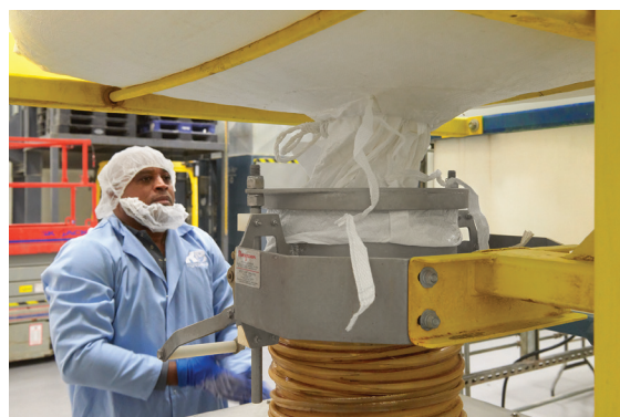
An operator secures the bag spout with a Spout-Lock® clamp ring positioned atop a Tele-Tube® telescoping tube that lowers, keeping the spout taut to promote flow and total evacuation.
