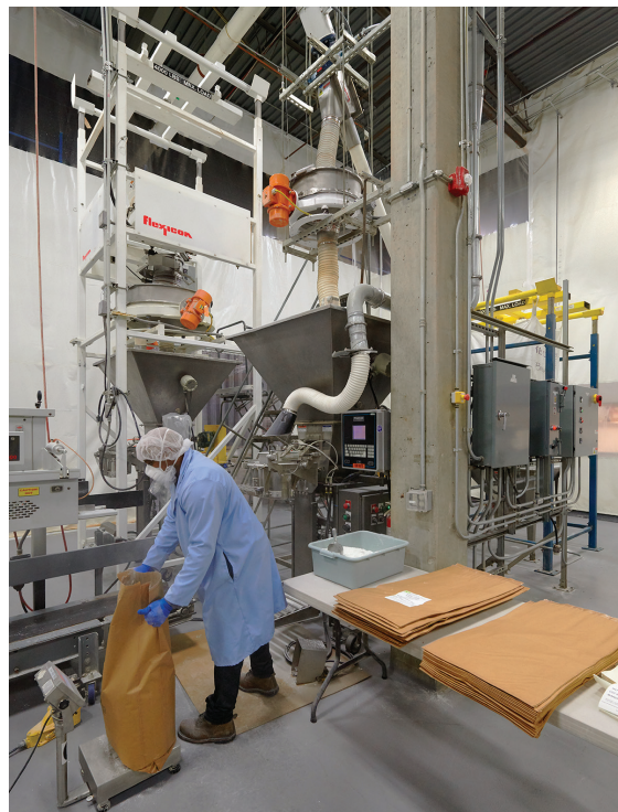
The company's second bulk bag discharger, with screener integrated into the frame, discharges blended material into a hopper above a packaging machine.
