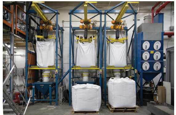
Bulk-Out® model BFC bulk bag dischargers unload three varieties of sand which flexible screw conveyors transport to the drum sanders. A cantilevered hoist and trolley lift each bag into the discharger frame.
