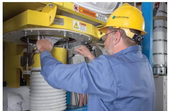
Once the bag spout is secured by the Spout-Lock® clamp ring, the Tele-Tube® telescoping tube applies constant downward tension as the bag empties and elongates to promote complete discharge and contain dust.
