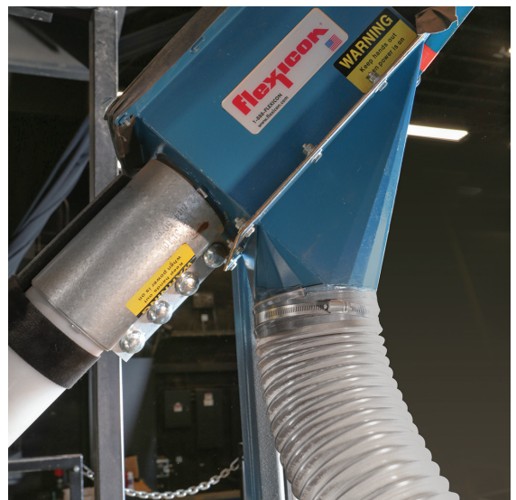
Cirque du Soleil’s production of KÀ at the MGM Grand in Las Vegas operates a cork cleaning system that removes dust, undersized/oversized particles and ferrous contaminants. Cork ‘sand’ flows from the stage to the basement, from where it conveyed pneumatically to a hopper that gravity discharges into a Flexicon Flexible Screw Conveyor, which in turn feeds the cork into a vibratory separator at controlled rates.
