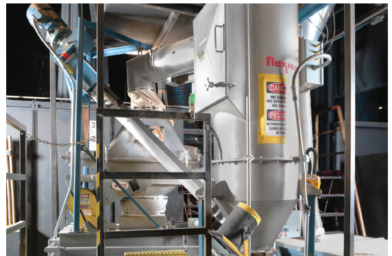
Cirque du Soleil’s production of KÀ at the MGM Grand in Las Vegas operates a cork cleaning system that removes dust, undersized/oversized particles and ferrous contaminants. Cork ‘sand’ flows from the stage to the basement, from where it conveyed pneumatically to a hopper that gravity discharges into a Flexicon Flexible Screw Conveyor, which in turn feeds the cork into a vibratory separator at controlled rates.
