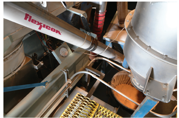
A shaftless screw rotating within an enclosed tube elevates the material and feeds it into the vibratory separator dust-free. The screw is driven beyond the point of discharge, avoiding material contact with bearings or lubricants.
