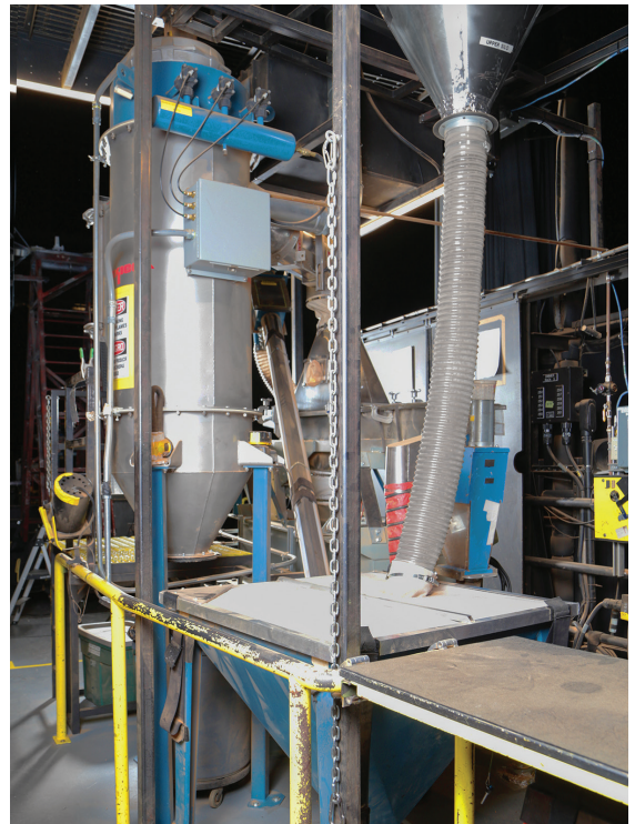
The flexible screw conveyor moves the wheat and oat materials together at the same speed with no separation.
