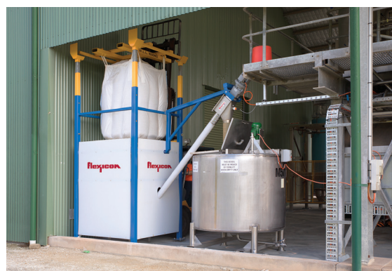
Tartaric acid gravity feeds from the bulk bag into the hopper and is transported by the flexible screw conveyor into the mixing tank.
