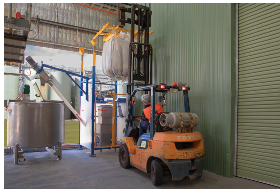
Operator secures bag to the lifting frame with Z-Clip™ bag strap holders, and then loads the frame and bag onto the main discharger frame.
