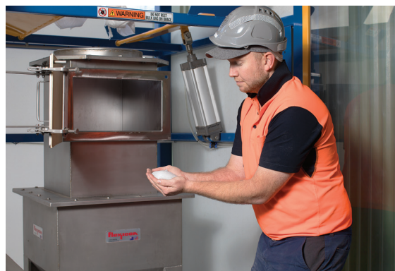
Operator pulls the bag spout into the bulk bag interface chute and unties the drawstring. A sealing ring, dust-tight door and filter sock contain dust.
