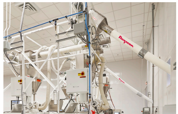
Flexible screw conveyors transfer ingredients from bulk bag dischargers in the warehouse, through a packaging room wall, and transfer into horizontal flexible screw conveyors that feed packaging machines. The screws are driven beyond the point of discharge, preventing product contact with seals or bearings.
