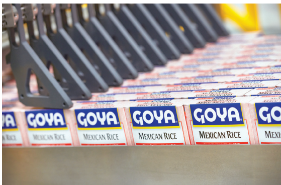
Filled and sealed packages of Goya's Spanish Rice and Mexican Rice proceed to a cartoning line.
