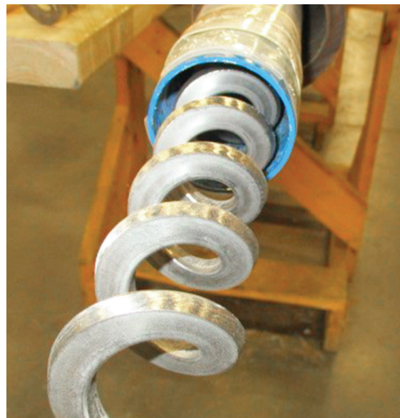
Specialized screw geometry enables the conveyor to move difficult materials.
