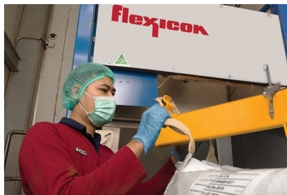
Operator attaches bulk bag to Z-Clip™ strap holders of a bag lifting frame.
