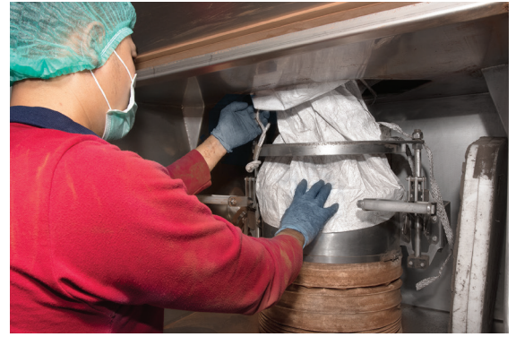
The clean side of the bag spout is secured to the clean side of the discharger by a Spout-Lock™ clamp ring. Constant downward tension is maintained by a Tele-Tube™ telescoping tube as the bag empties and elongates.
