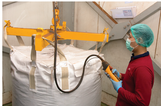
Operator attaches bulk bag to Z-Clip™ strap holders of a bag lifting frame.
