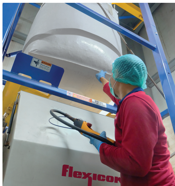
An electric hoist and trolley on a cantilevered I-beam enable an operator to raise and position the bag using a pendant, eliminating the need for a forklift.
