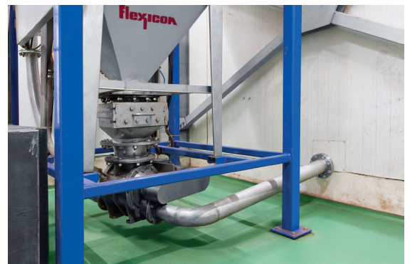
The clean side of the bag spout is secured to the clean side of the discharger by a Spout-Lock™ clamp ring. Constant downward tension is maintained by a Tele-Tube™ telescoping tube as the bag empties and elongates.
