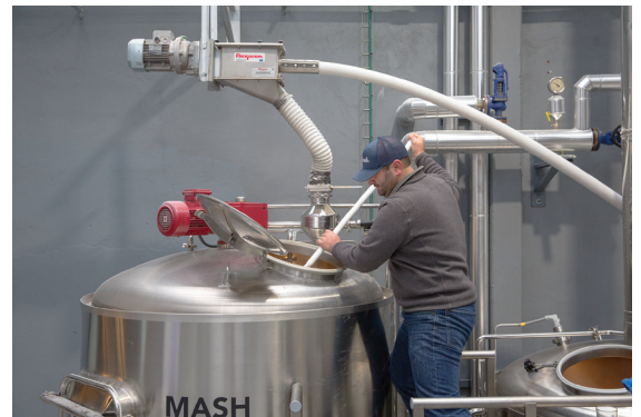
The drive motor of the flexible screw conveyor is located beyond the discharge point, preventing material contact with seals or bearings.
