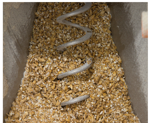
The conveyor's flexible screw moves the wheat-oat blend from the hopper into the conveyor's tube. The spiral has ample room between the tube walls to avoid grinding of the material.
