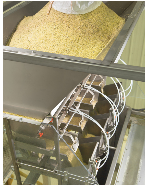
Hemp hearts flow from the bulk bag discharger into a scale and to packaging on the level below.
