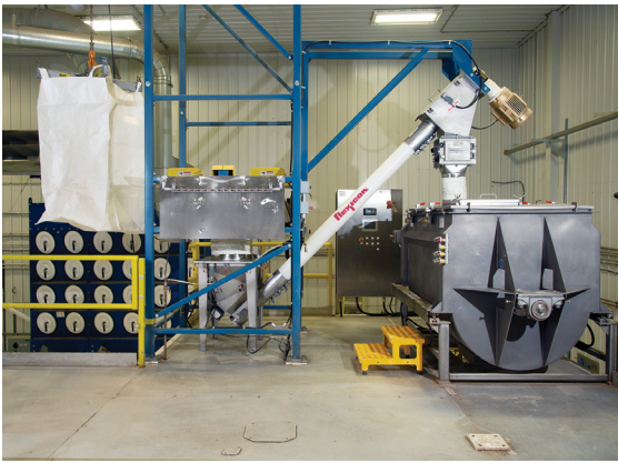
The BFC model bulk bag discharger, equipped with cantilevered I-beam, hoist and trolley, lifts the bulk bag from the level below.
