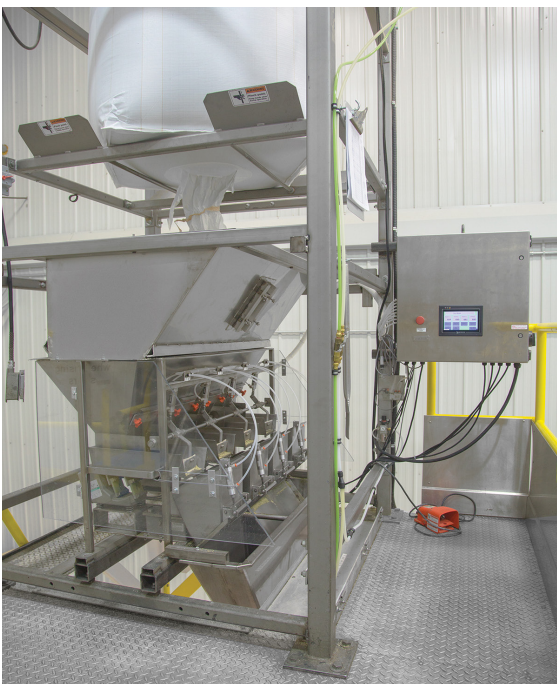
The bag spout interface prevents dusting and promotes flow by virtue of a Spout-Lock® clamp ring and Tele-Tube® telescoping tube. Promoting total evacuation from the bag are Flow-Flexer bag activators.
