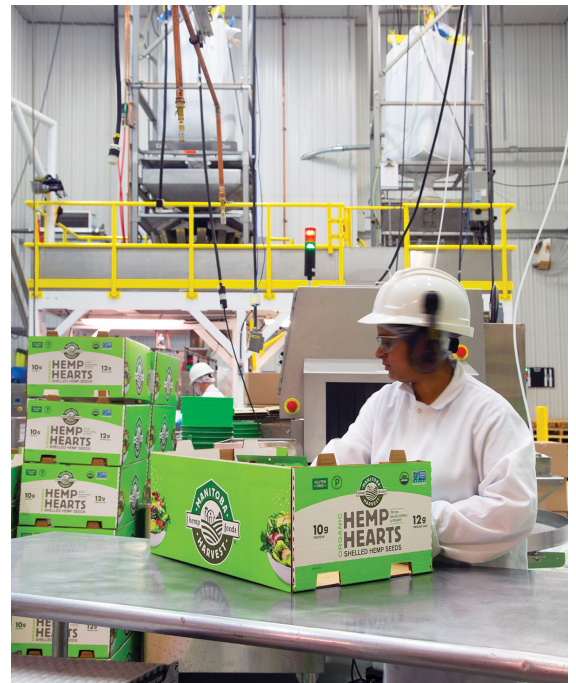
Hemp hearts flow from the bulk bag discharger into a scale and to packaging on the level below.
