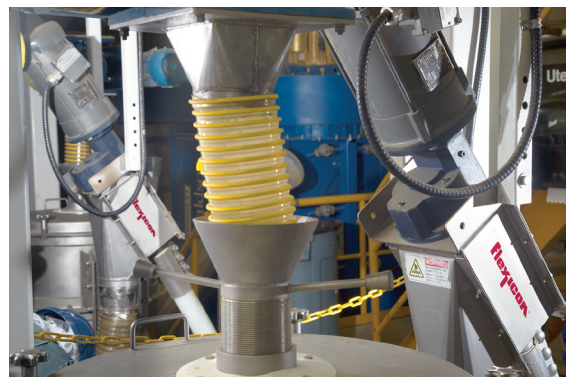
Each pair of interconnected flexible screw conveyors discharges processed material into a separator for further processing.
