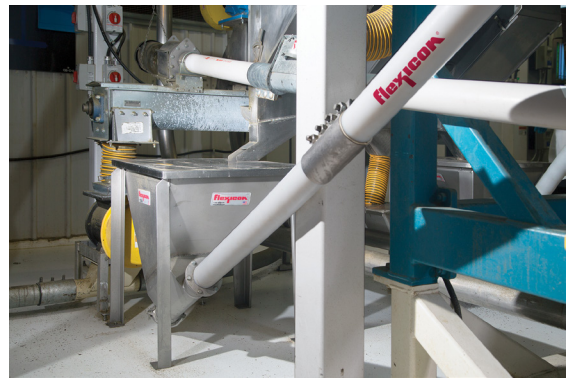
Two 30 ft (9 m) long conveying systems each consist of a 10 ft (3 m) long flexible screw conveyor that connects to the charging adaptor of a 20 ft (6 m) long flexible screw conveyor.
