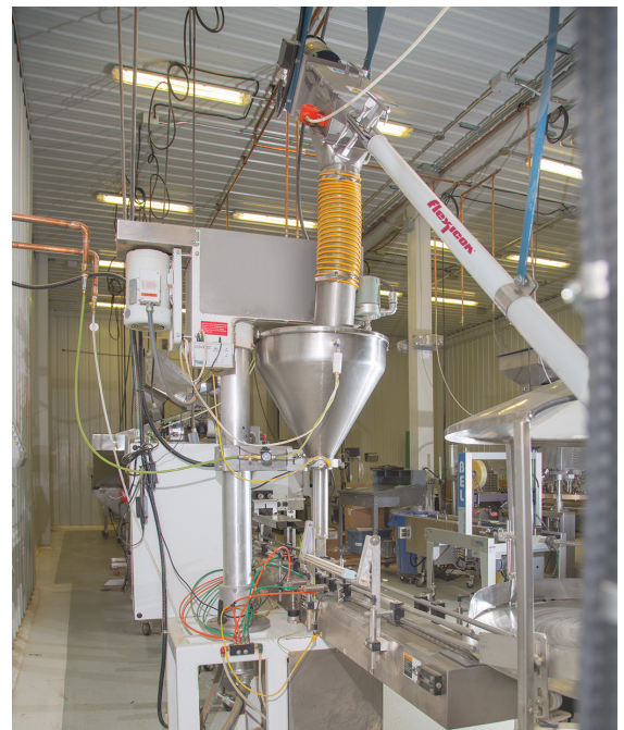
Final milled muscovite material has gone through size reduction, pneumatic conveying, drying and sieving steps.
