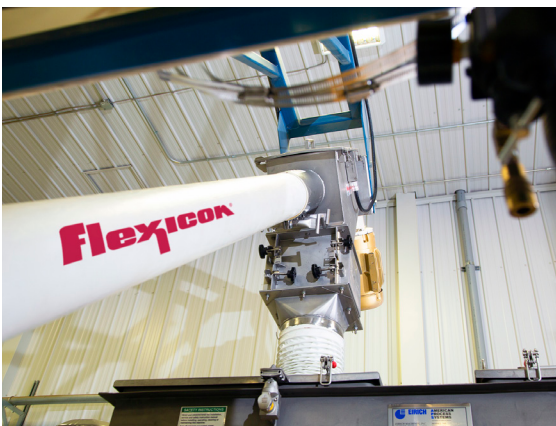
The bulk bag discharger and flexible screw conveyor gently feed the blender which mixes protein powder and other ingredients.
