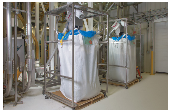
Caster-mounted hoppers and flexible screw conveyors transport work-in-process and bulk shipment material into each bulk bag.
