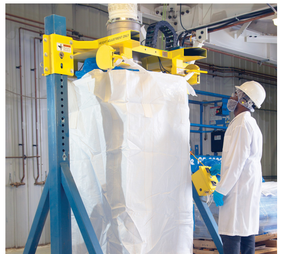
Twin Centerpost bulk bag filler receives material through a sealed chute from the blender on the level above. The operator attaches the bag spout to the inflatable collar on the fill head. A blower inflates the bag prior to filling, eliminating creases and pre-shaping the bag for stability
