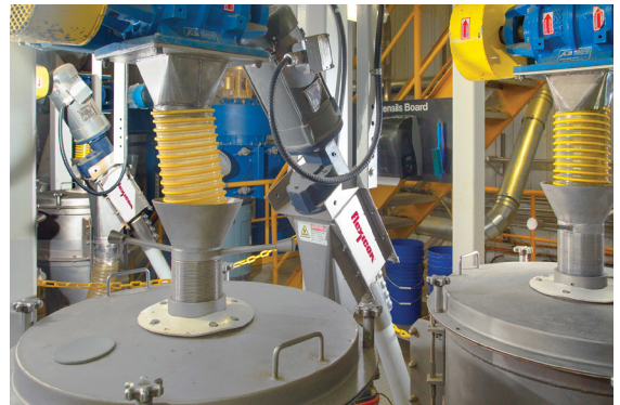
Two 30 ft (9 m) long conveying systems each consist of a 10 ft (3 m) long flexible screw conveyor that connects to the charging adaptor of a 20 ft (6 m) long flexible screw conveyor.
