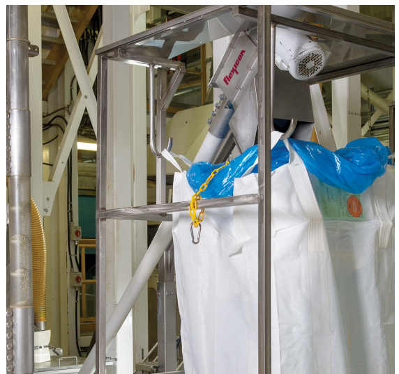
Each pair of interconnected flexible screw conveyors discharges processed material into a separator for further processing.
