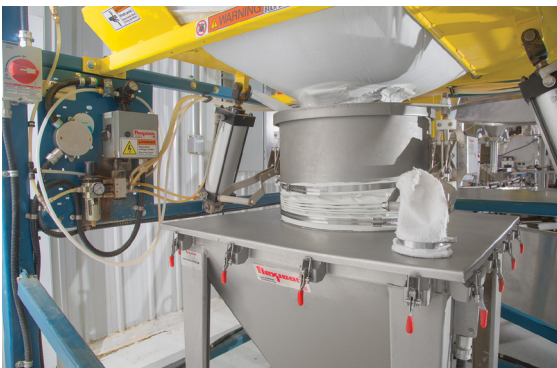
The bag spout interface prevents dusting and promotes flow by virtue of a Spout-Lock® clamp ring and Tele-Tube® telescoping tube. Promoting total evacuation from the bag are Flow-Flexer bag activators.
