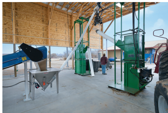
Biomass is discharged from the flexible screw conveyor into a wye diverter, which feeds two balers.
