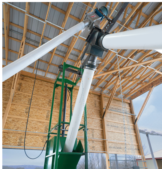
The flexible screw conveyor’s motor drive is positioned beyond the material discharge point, preventing product contact with seals or bearings.
