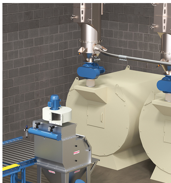
Under PLC control, the pneumatically-actuated diverter valves of three filter receivers open and close in sequence. The PLC also starts and stops rotary airlock valves according to signals received from high and low level sensors of the mixing tank surge hoppers.
