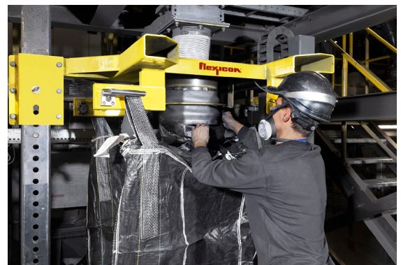
At the Twin-Centrepost bulk bag filler, the operator secures the bag spout to the fill head with inflatable collar to assure dust-free filling. The height-adjustable fill head accommodates various bulk bag sizes.
