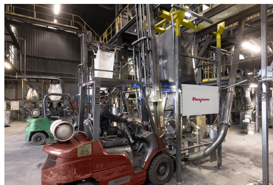
A fork truck loads the liftring cradle with bulk bag into receiving cups atop the discharger posts.
