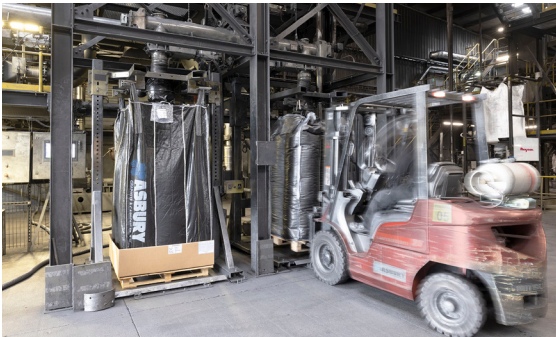
From the silo above, milled graphite continuously fills into a pair of bulk bag fillers.
