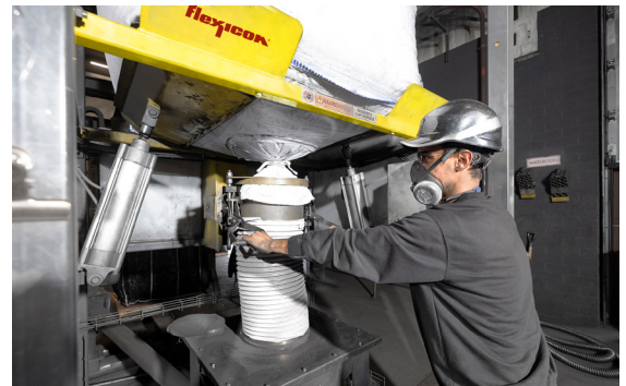
A SPOUT-LOCK® clamp ring positioned atop a TELE-TUBE® telescoping tube applies constant downward tension as the bag empties and elongates for full and dust-free evacuation.
