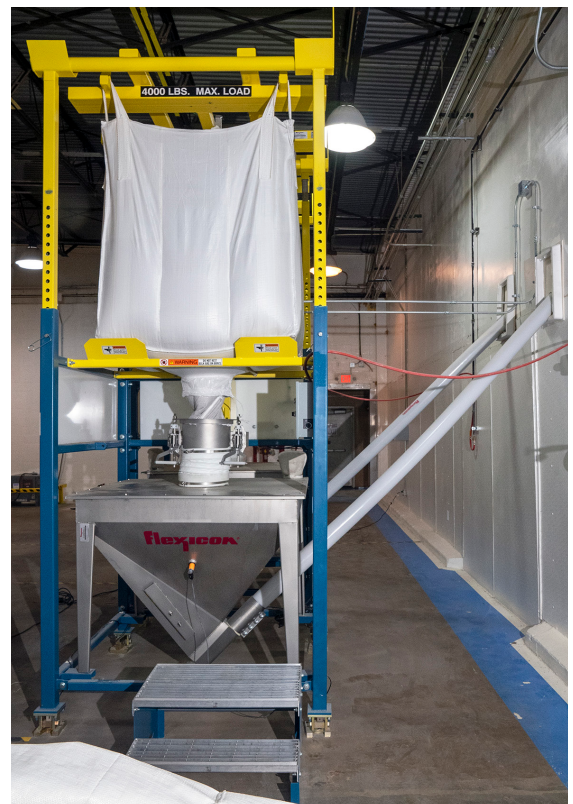
Two forklift-loaded bulk bag dischargers feed lentils to each floor hopper from which a flexible screw conveyor transports the lentils through the wall into the Packaging Room.
