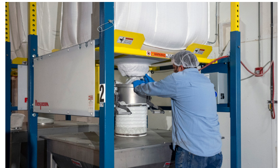
Two forklift-loaded bulk bag dischargers feed lentils to each floor hopper from which a flexible screw conveyor transports the lentils through the wall into the Packaging Room.
