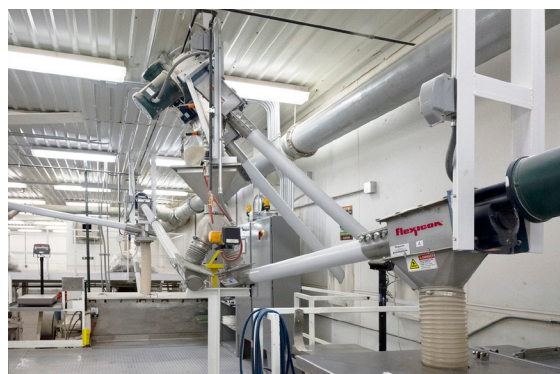
In the Packaging Room, two flexible screw conveyors move lentils from the two bulk bag dischargers outside to a transition hopper from which four interconnected flexible screw conveyors deliver lentils to four mixers.
