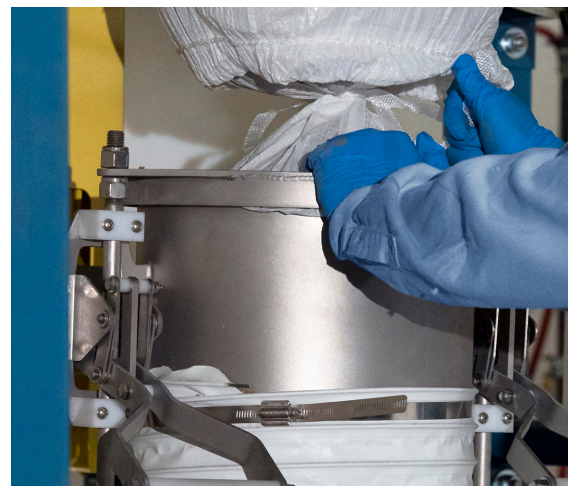
The SPOUT-LOCK® clamp ring positioned atop the TELE-TUBE® telescoping tube applies constant downward tension as the bag empties and elongates for full and dust-free evacuation.
