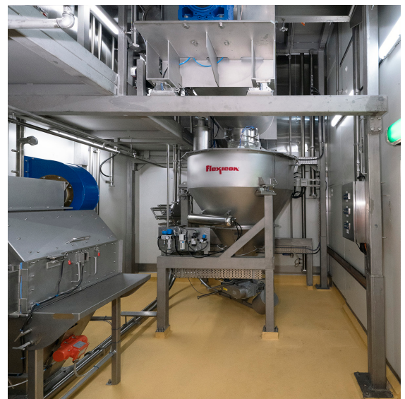
Each batch is accumulated in this filter receiver, which gravity discharges into a mixer.
