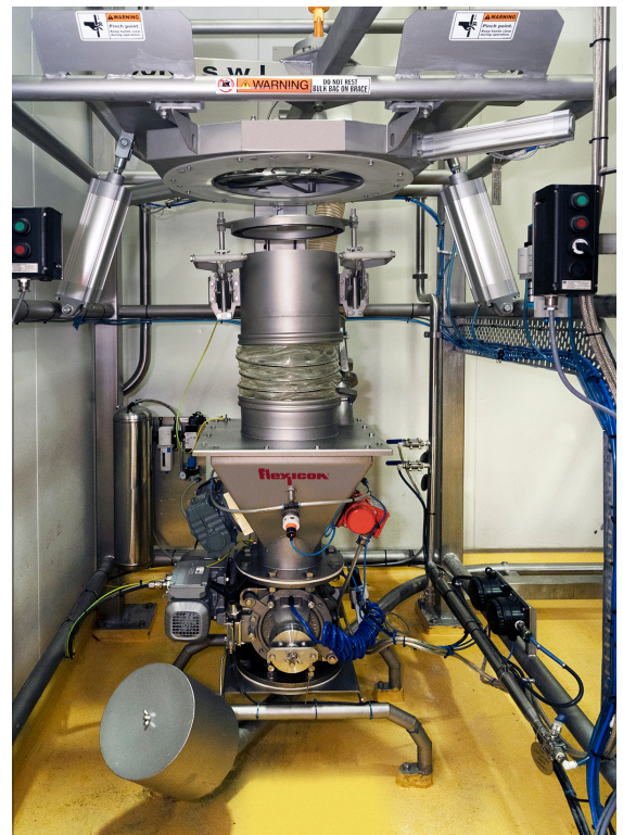
Flow-Flexer™ bag activator plates driven by pneumatic cylinders (top) raise and lower opposite bottom sides of the bag to promote flow, as a Spout-Lock™ clamp ring atop a Tele-Tube™ telescoping tube applies downward tension as the bag empties and elongates, promoting complete discharge. The rotary airlock valve beneath the hopper meters material into the pneumatic line.
