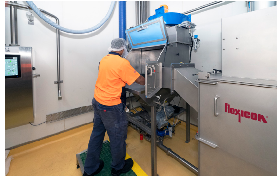
Small bags containing low volume ingredients are emptied into the bag tip station and metered into a pneumatic line through a rotary airlock valve. The bag compactor, at right, compresses empty bags for dust-free disposal.
