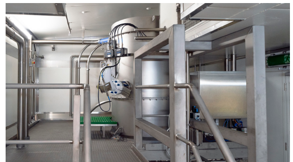
Each batch is accumulated in this filter receiver, which gravity discharges into a mixer.
