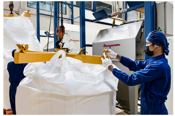
Operator attaches bulk bag to Z-Clip™ strap holders of the bag lifting frame.
