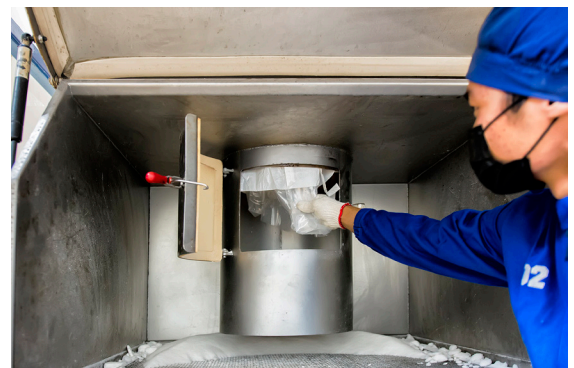
Operator pulls the bag through the iris valve, which closes around the spout, allowing gradual opening and dust-free material flow.
