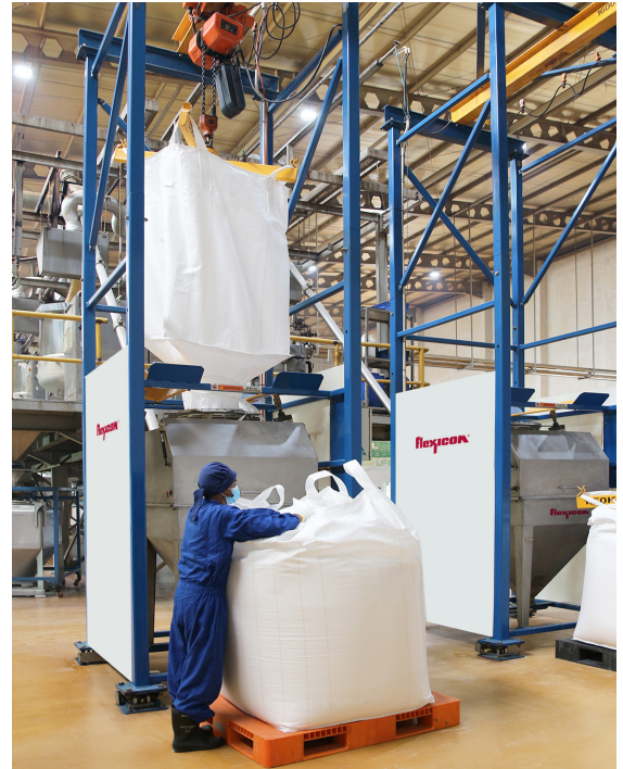
Operator attaches bulk bag to Z-Clip™ strap holders of the bag lifting frame.
