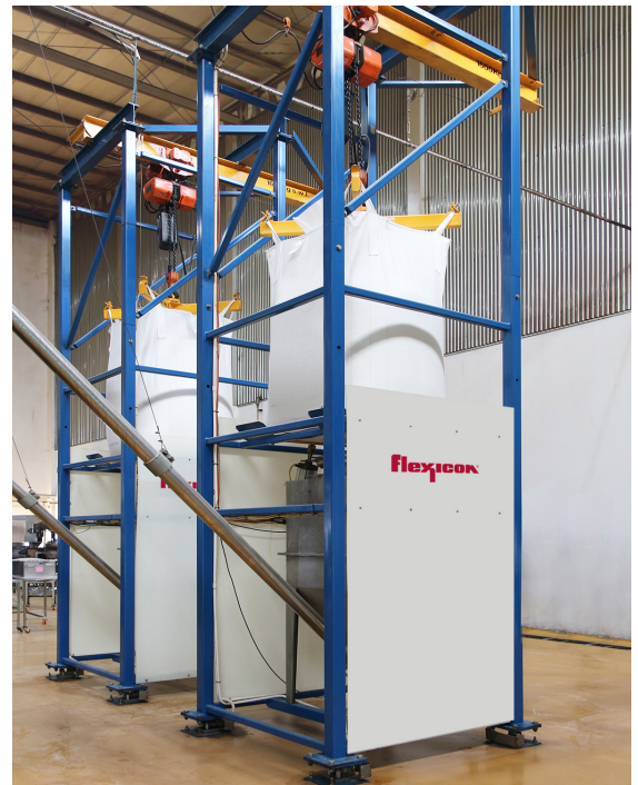
A cantilevered I-beam, hoist and trolley load a bulk bag into each discharger frame without need of a forklift.
