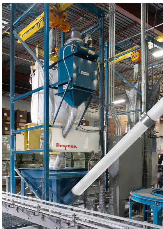
Each bulk bag discharger is equipped with a BAG-VAC® dust collector that contains dust within the sealed system and collapses empty bags prior to tie-off.
