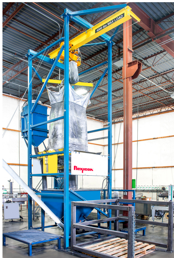
This bulk bag discharger and flexible screw conveyor feed a graphite packaging line that fills 1 and 5 lb (0.45 and 2.25 kg) containers.
