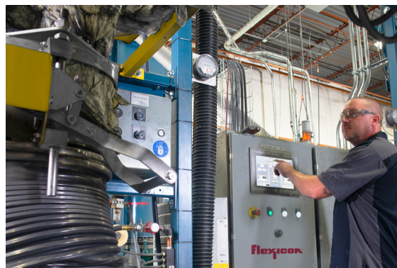
The gain-in-weight control system enables operators to specify graphite-talc ratios and batch weights.
