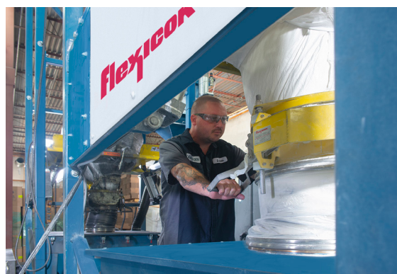
As the bag empties and elongates, the TELE-TUBE® telescoping tube exerts continuous downward tension on the SPOUT-LOCK® clamp ring and bag spout, promoting flow and evacuation.
