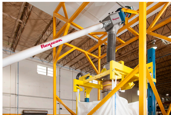
Flexible screw conveyor transfers ground coffee from the grinder through downspouting to the bulk bag filler.
