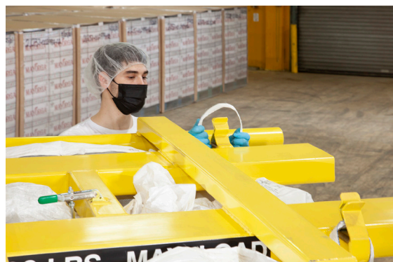
At floor level, an operator attaches bulk bag straps to Z-Clip™ strap holders of a bag lifting frame held in position by a forklift.
