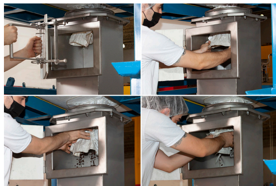
Operator opens access door and pulls the bag outlet spout through the sealing ring before untying the spout's drawstring.
