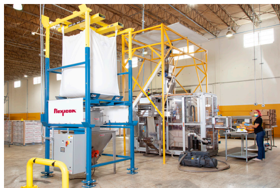
Bulk bag discharger unloads ground coffee into a floor hopper, charging a flexible screw conveyor that feeds the packaging machine.
