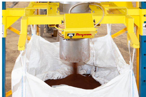
Bag strap hooks hold the bag open and stabilize it during filling.
