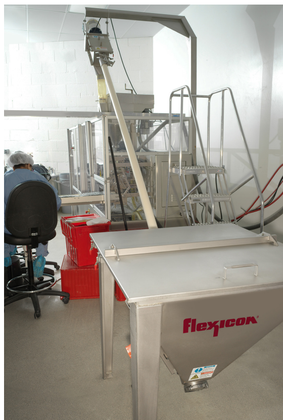
The enclosed hopper and flexible screw conveyor assure dust-free transfer. All product contact surfaces are of stainless steel.
