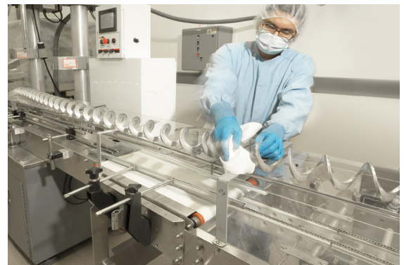
The flexible screw conveyor tube and spiral are disassembled and cleaned at regular intervals.
