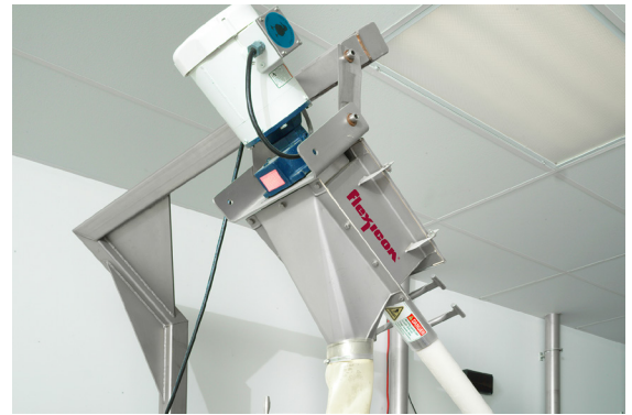
The conveyor screw is driven above the point of discharge, preventing material contact with bearings or seals.
