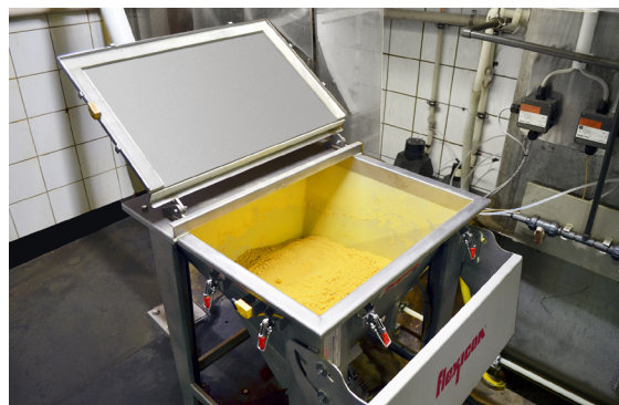
The 110 L (3.9 cu ft) capacity hopper, with fold-down support tray and hinged lid, is equipped with a mechanical agitator to reduce agglomerates, promoting flow into the conveyor's charging adapter.
