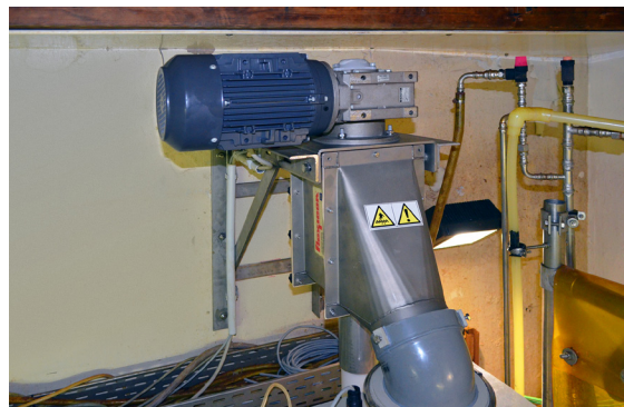
The flexible screw is driven by a 2.2 kW (2.95 hp), 1425 rpm IP65 electric motor beyond the material discharge point, precluding material contact with seals.
