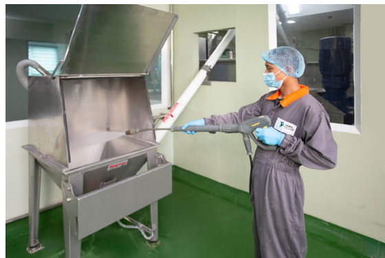
The operator removes and cleans the flexible screw conveyor's spiral and cleans the hopper with high pressure water.
