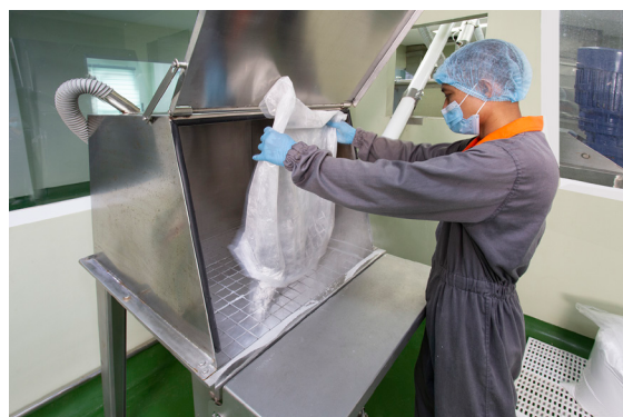
A fold-down support tray provides a staging area for operators to position and slit bags before dumping. The 140 L (5cu ft) capacity hopper has steep sides promoting flow of semi-free-flowing materials to the charging adapter for the flexible screw conveyor.
