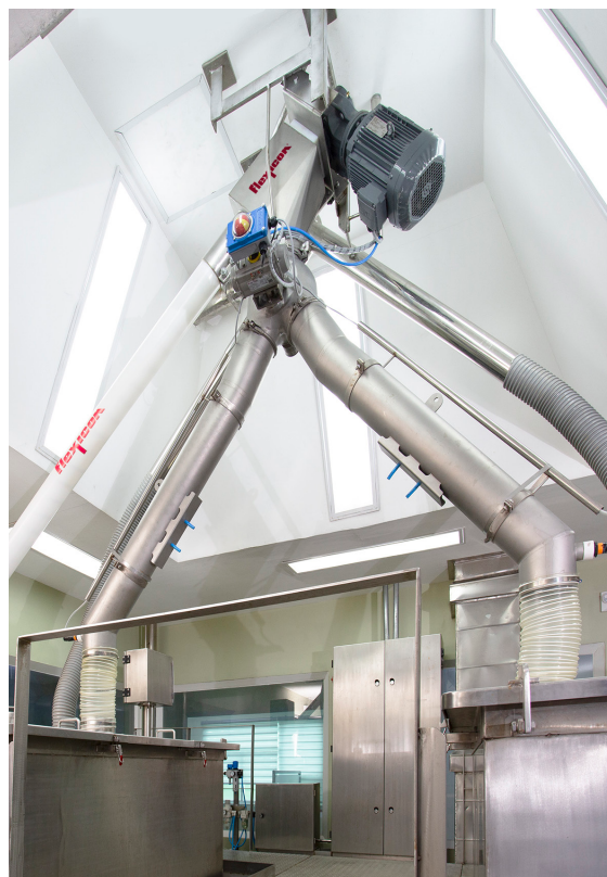
A fold-down support tray provides a staging area for operators to position and slit bags before dumping. The 140 L (5cu ft) capacity hopper has steep sides promoting flow of semi-free-flowing materials to the charging adapter for the flexible screw conveyor.
