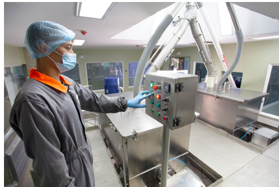
The flexible screw conveyor discharges through a wye diverter that diverts material into either of two 1000kg (1.1 U.S. ton) ribbon blenders. The conveyor is driven by an electric motor positioned beyond the discharge point, preventing contact with seals or bearings.
