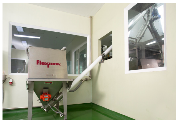
The floor hopper and control panel are housed in a separate room from the blending operation, with the flexible screw conveyor passing through an opening in the adjoining wall. The IP65 variable speed control panel with human-machine-interface allows easy operation of the conveyor and actuation of the diverter valve in the blending room.
