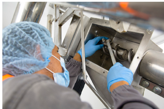
The flexible screw conveyor discharges through a wye diverter that diverts material into either of two 1000kg (1.1 U.S. ton) ribbon blenders. The conveyor is driven by an electric motor positioned beyond the discharge point, preventing contact with seals or bearings.
