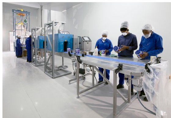
View from both ends of automated packaging line, with bulk bag discharger and packaging machine. It is one of seven identical lines.
