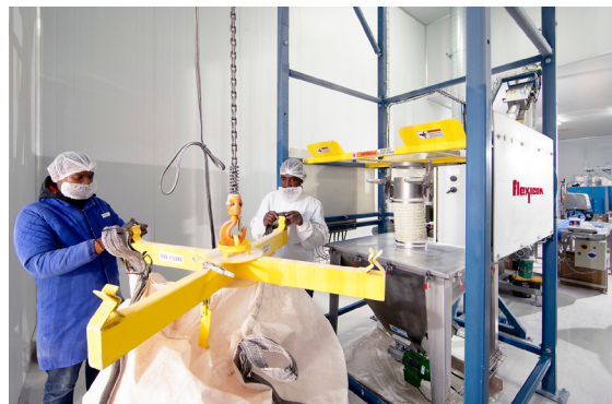
View from both ends of automated packaging line, with bulk bag discharger and packaging machine. It is one of seven identical lines.
