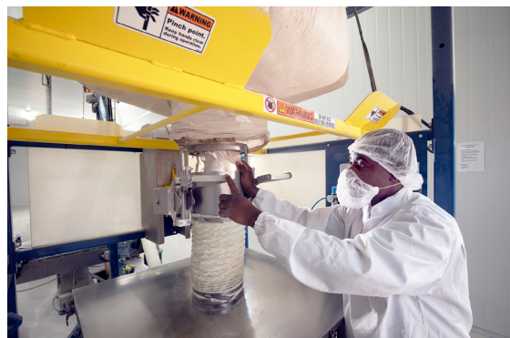
The bag spout is attached to a SPOUT-LOCK ™ clamp ring atop a TELE-TUBE ™ telescoping tube which applies downward tension for complete discharge into the hopper.
