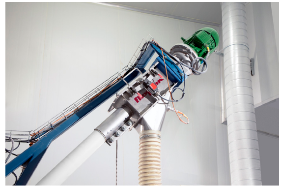
The flexible screw conveyor's drive is located beyond the point of discharge, preventing material contact with seals or bearings.
