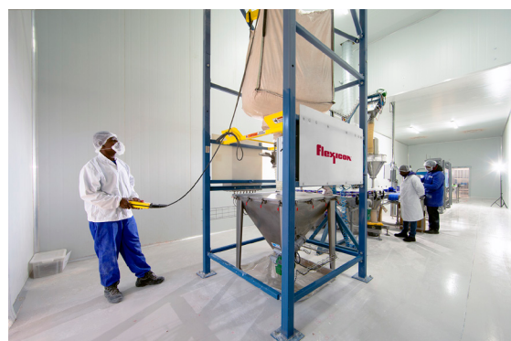
Operators attach bag loops to the lifting frame with Z-CLIP ™ bag strap holders and hoist it into the discharger using a pendant.
