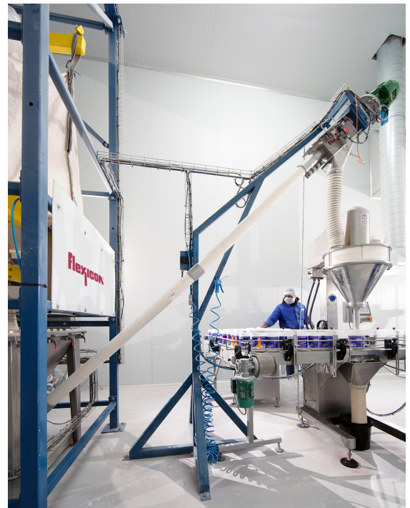
Operator initiates a bulk transfer cycle. PLC control provides for continuous filling and accurate package weights.
