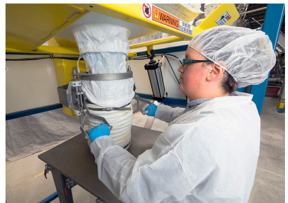
The operator connects the bag spout to the Spout-Lock® clamp ring and Tele-Tube® telescoping tube, which maintains constant downward tension on the bag as it empties and elongates, promoting flow.
