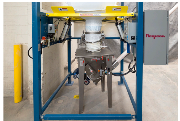
The hopper is fitted with internal agitators and a wall-mounted vibrator to promote the flow of seasonings into the conveyor's charging adapter.
