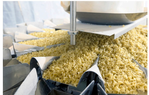
Pasta feeds into the pouch filler below after the seasonings have been added.
