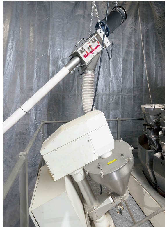
The conveyor screw is driven beyond the point of discharge, preventing material contact with bearings or seals.
