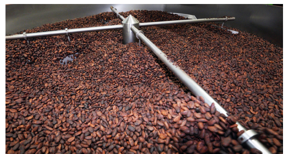
Roasted beans cool in the tray before being conveyed to the winnower and subsequent processing into cocoa liquor.
