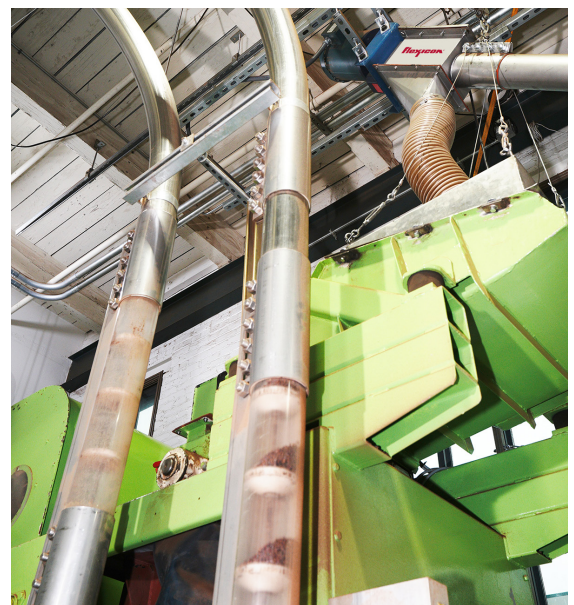
Clear section of the tubular cable conveyor (TCC) allows visual monitoring of performance and pocket fill percentage.
