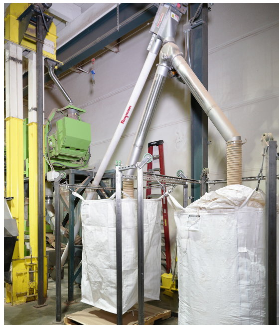
Raw cocoa beans from the destoner-cleaner are transported by the flexible screw conveyor through a wye diverter and into the bulk bags.
