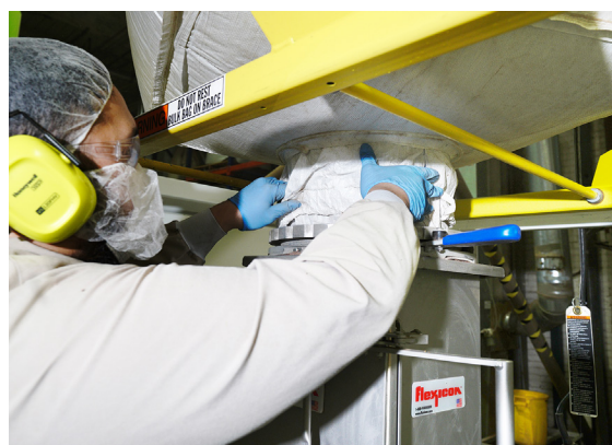
The operator closes the iris valve, securing the bag spout and supporting dust.
