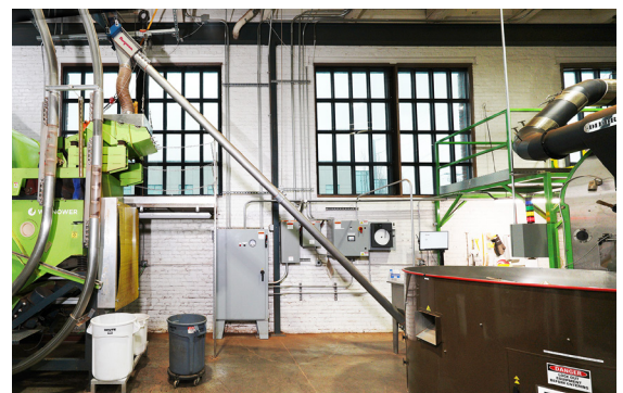
From the roaster, the flexible screw conveyor transports cooked beans to the winnower which separates the bean shells from the nibs.
