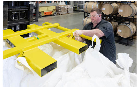
A removable lifting frame is attached to bag straps and forklifted onto cradle cups atop the discharger.
