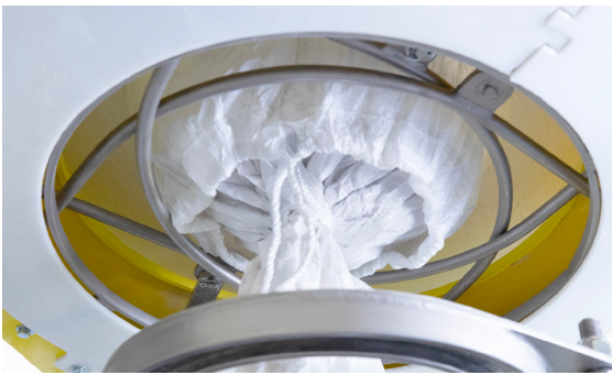
At the bag spout interface, a POWER-CINCHER® flow control valve cinches the bag spout prior to releasing the drawstring. The valve can then be opened gradually to avoid bursts of material into the hopper, or closed to allow retying of partially empty bags.
