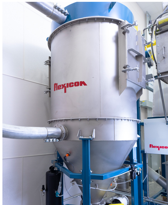
The pneumatic line circuit terminates at a filter-receiver that separates carry-over material and returns it to the pneumatic feed line, eliminating waste.
