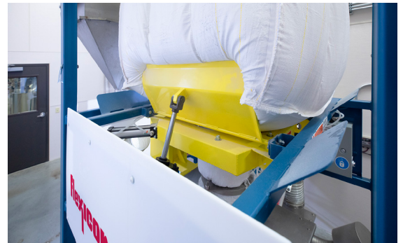
A TELE-TUBE® telescoping tube maintains continuous downward tension on the bag as it empties and elongates, promoting flow and complete discharge.
