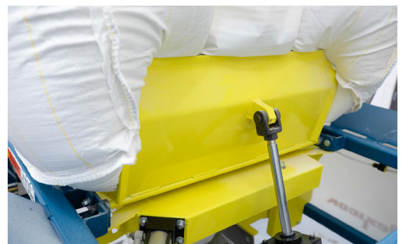
FLOW-FLEXER® bag activators press on opposite bottom sides of the bag to break up clumps of grain that formed during shipment and storage, directing all of the grain through the spout.
