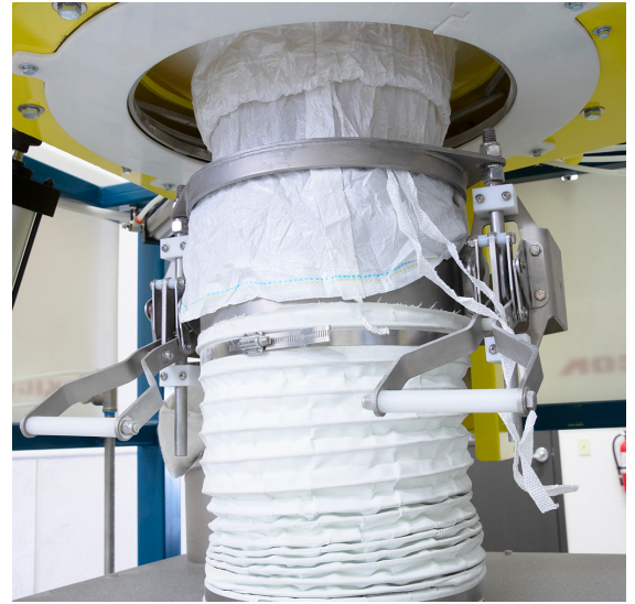
A TELE-TUBE® telescoping tube maintains continuous downward tension on the bag as it empties and elongates, promoting flow and complete discharge.
