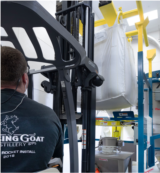
The lifting frame with bag intact, is lifted onto the frame's upper cradle.
