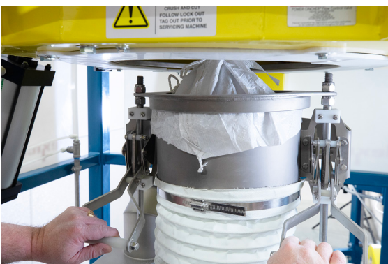
A SPOUT-LOCK® clamp ring secures the clean side of the spout to the clean side of the equipment.
