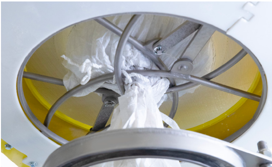
The lifting frame with bag intact, is lifted onto the frame's upper cradle.
