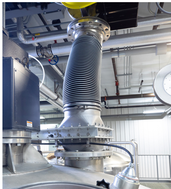
Precise batch weights are fed to each of three cookers, with no residual in the conveying line.
