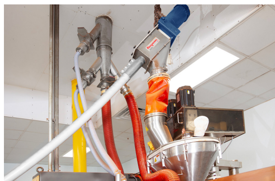
Material discharges from the flexible screw conveyor upstream of the drive motor, precluding contact with bearings or seals.
