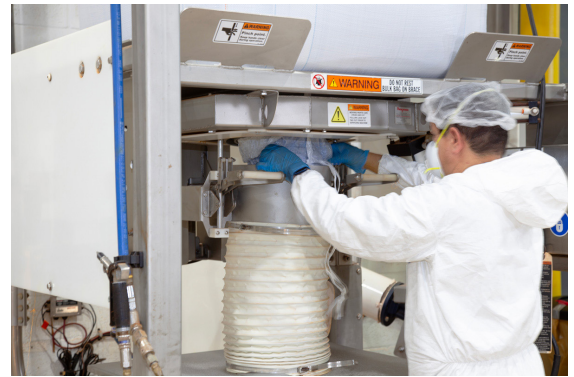
A SPOUT-LOCK® clamp ring makes a dust-tight connection while a TELE-TUBE® telescoping tube applies downward tension on the bag, promoting flow and evacuation.
