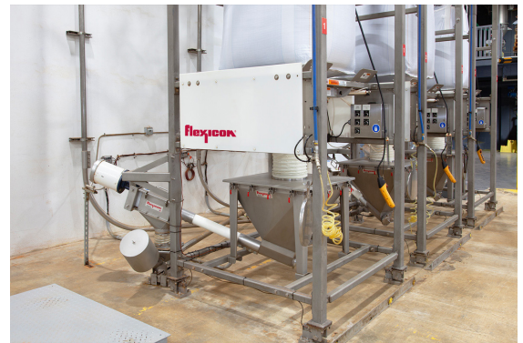
A flexible screw conveyor (foreground) feeds seasoning into the pickup adapter of a 55 ft (17 m) pneumatic conveying line routed to a blender.
