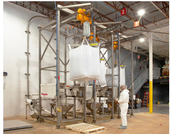
The operator unties the bag spout, allowing sugar to flow into the floor hopper and through a rotary valve into the PNEUMATI-CON® pneumatic conveying line. On the left and right, flexible connections vent dust to filter socks.
