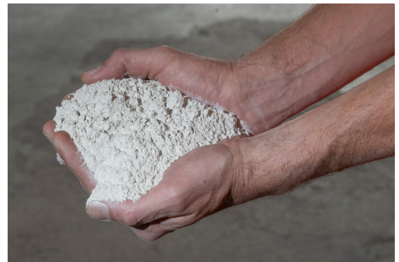
Final milled muscovite material has gone through size reduction, pneumatic conveying, drying and sieving steps.
