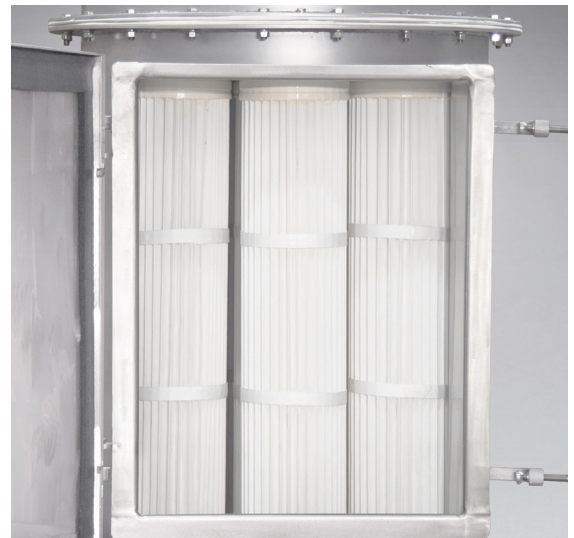
The filter receiver separates sugar from the air stream through filter media. Reverse-pulse jet cleaning dislodges accumulated dust for continuous separation of material.
