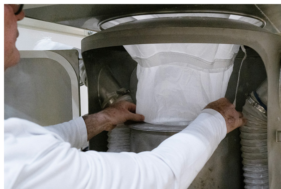
The operator unties the bag spout, allowing sugar to flow into the floor hopper and through a rotary valve into the PNEUMATI-CON® pneumatic conveying line. On the left and right, flexible connections vent dust to filter socks.
