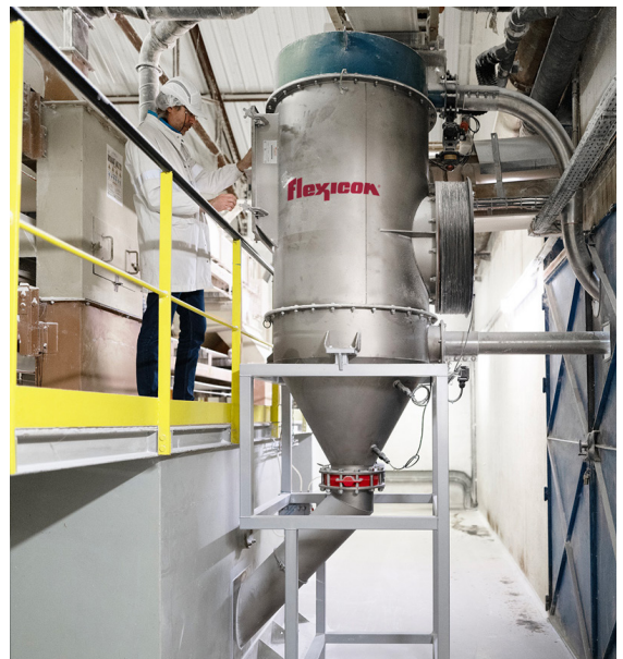
Sugar Fed from Bulk Bags Pneumatically at Tereos Artenay
