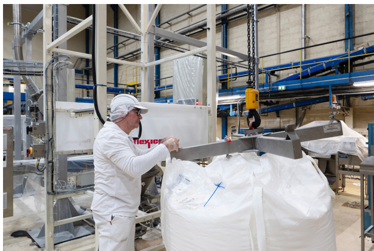
Operator attaches bulk bag to lifting frame with Z-CLIP™ bag strap holders before hoisting the bag into the discharger frame.
