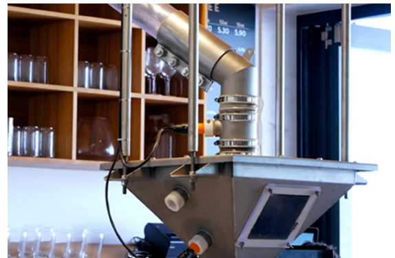
Customers watch roasted beans gravity discharge from the Tubular Cable Conveyor through clear tubing into a surge hopper.
