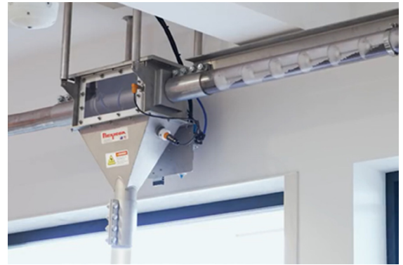
The Tubular Discharge Valve is opened to dispense the beans into a grinder or closed to allow the beans to travel on to the whole bean packaging station.
