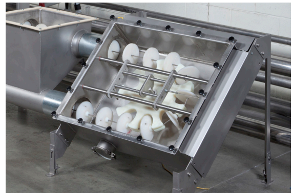
The polymer discs and cable are driven by a wheel at one end of the circuit and kept under tension by a wheel at the opposite end.
