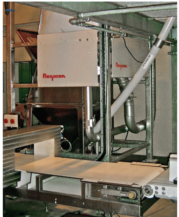
This bulk bag discharger with integral flexible screw conveyor moves malt from bulk bags to the bagging line.
