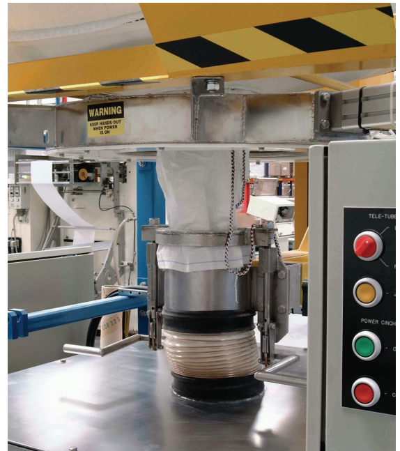
SPOUT-LOCK® clamp ring and TELE-TUBE® telescoping tube allow quick, dust-free connections between bag spout and hopper and elongate bag as it empties to promote flow.
